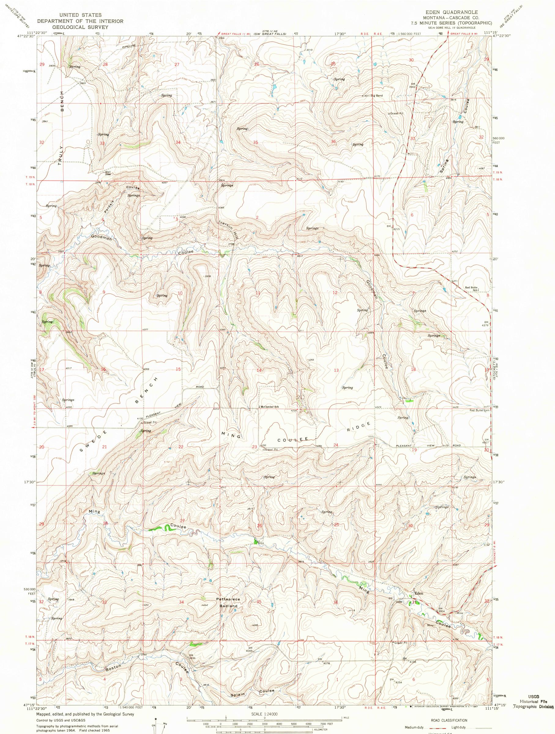
Polyconic projection. 1927 North American datum 0°14' 4 MILS 10,000-foot grid based on Montana coordinate system, central zone 1000-meter Universal Transverse Mercator grid ticks, zone 12, shown in blue UTM GRID AND 1965 MAGNETIC NORTH DECLINATION AT CENTER OF SHEET Fine red dashed lines indicate selected fence lines
