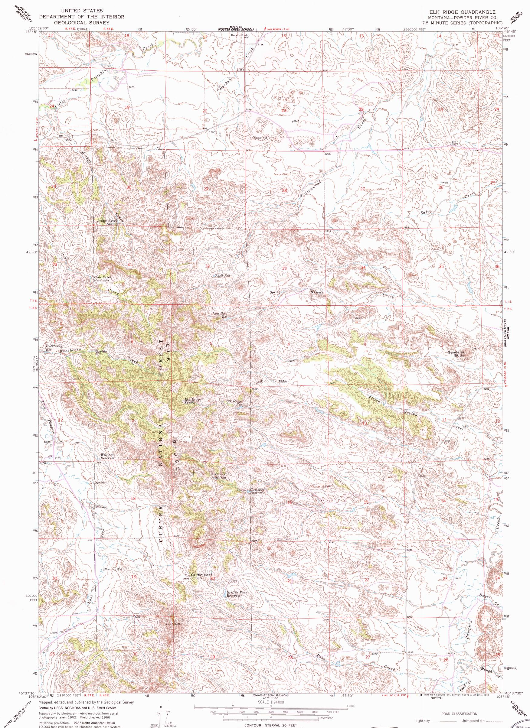
Polyconic projection. 1927 North American Datum 10,000-foot grid based on Montana coordinate system, south zone 1000-meter Universal Transverse Mercator grid ticks, zone 13, shown in blue Fine red dashed lines indicate selected fence lines To place on the predicted North American Datum 1983 move the projection lines 6 meters north and 45 meters east as shown by dashed corner ticks There may be private inholdings within the boundaries of the National or State reservations shown on this map
