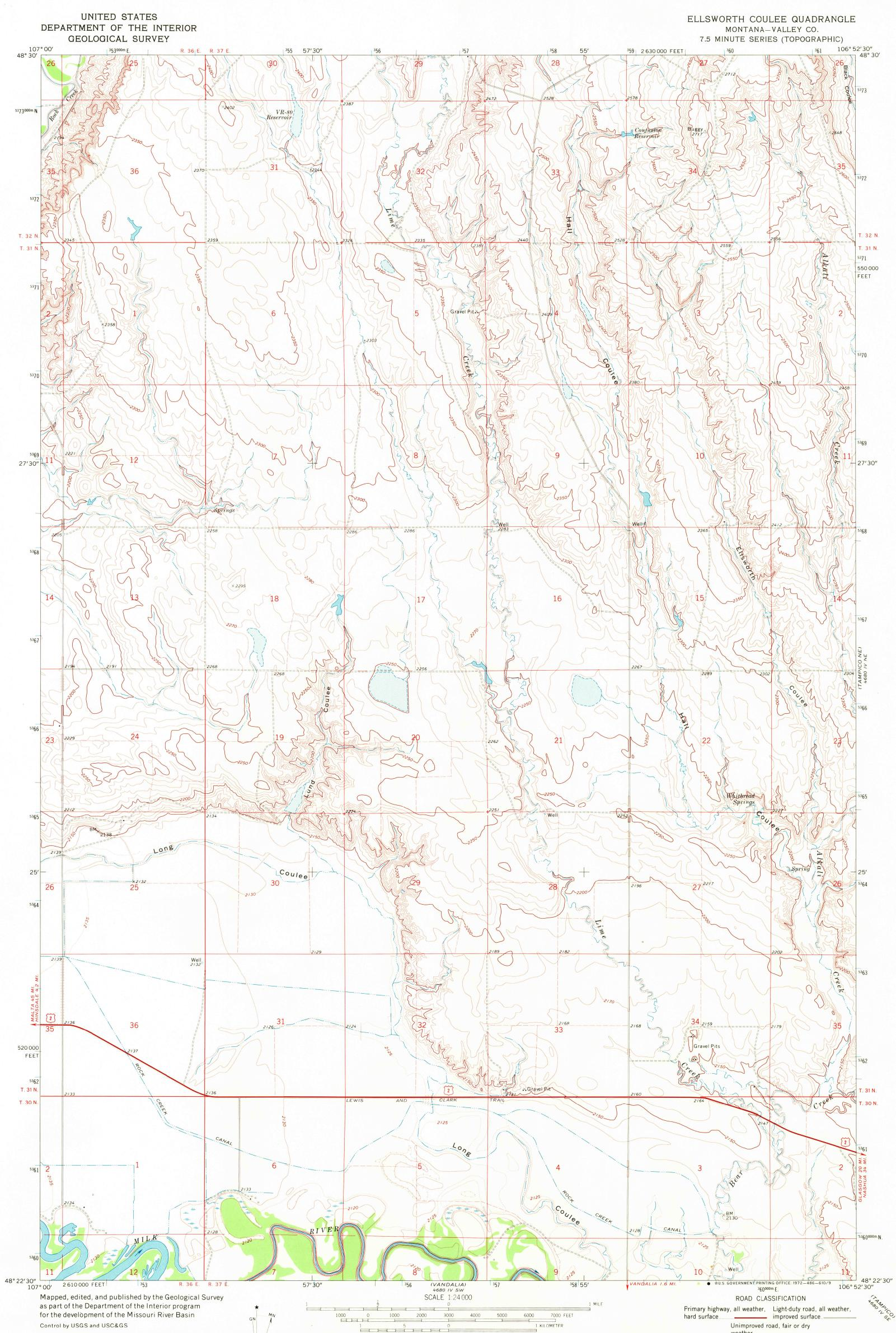
Topography by photogrammetric methods from aerial photographs taken 1967. Field checked 1969 Polyconic projection. 1927 North American datum 10,000-foot grid based on Montana coordinate system, north zone 1000-meter Universal Transverse Mercator grid ticks, zone 13, shown in blue Fine red dashed lines indicate selected fence lines
