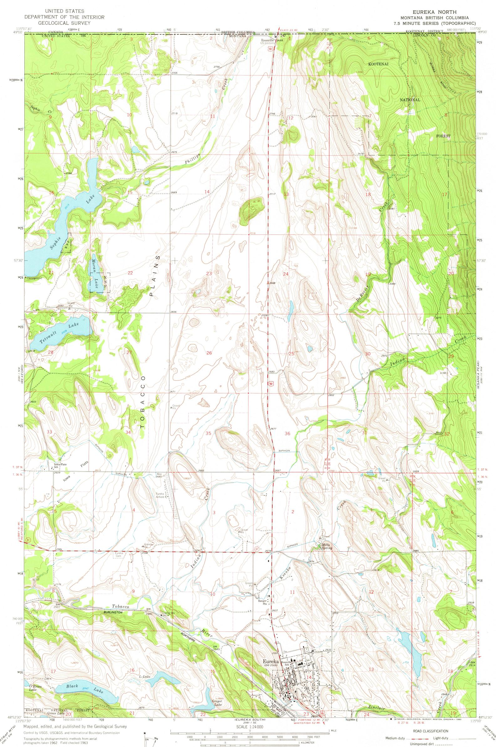
Polyconic projection. 1927 North American datum 10,000-foot grid based on Montana coordinate system, north zone 1000-meter Universal Transverse Mercator grid ticks, zone 11, shown in blue
