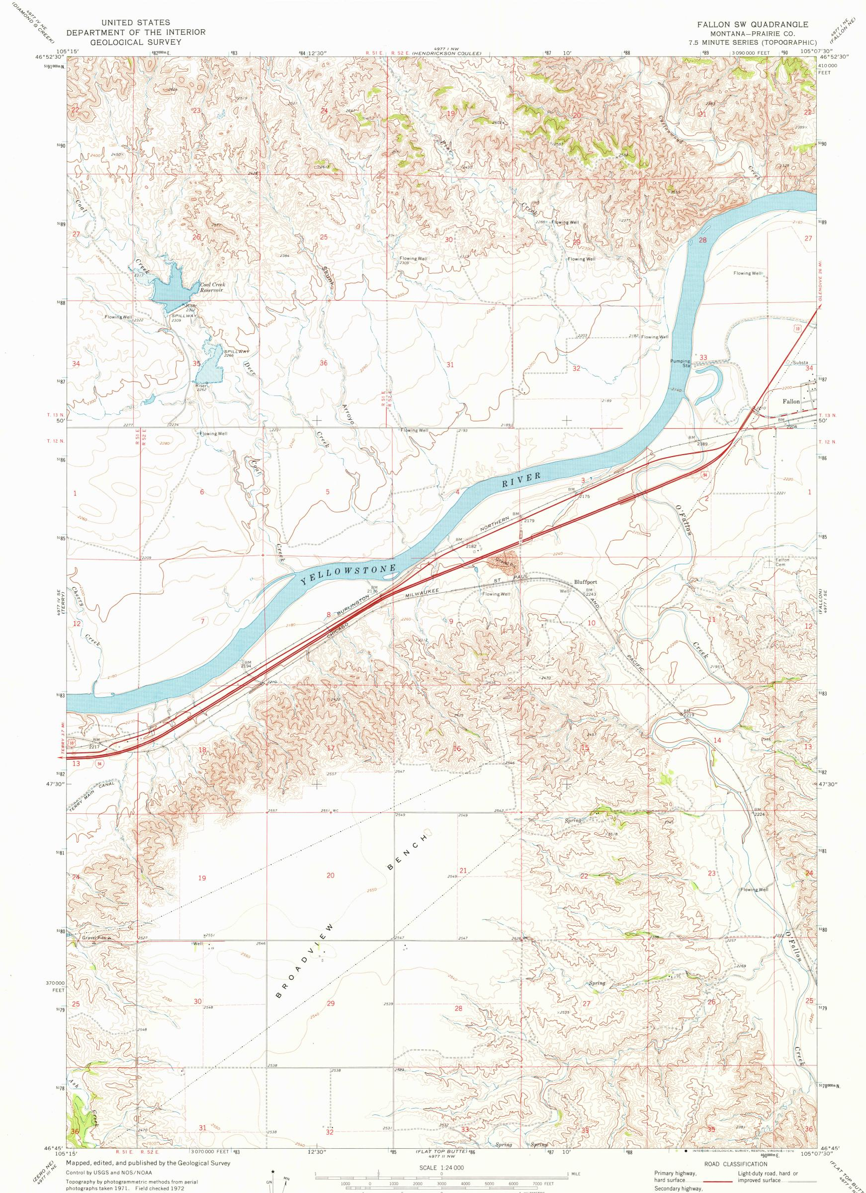
Projection and 10,000-foot grid ticks: Montana coordinate system, central zone (Lambert conformal conic) 1000-metre Universal Transverse Mercator grid ticks, zone 13, shown in blue. 1927 North American datum
