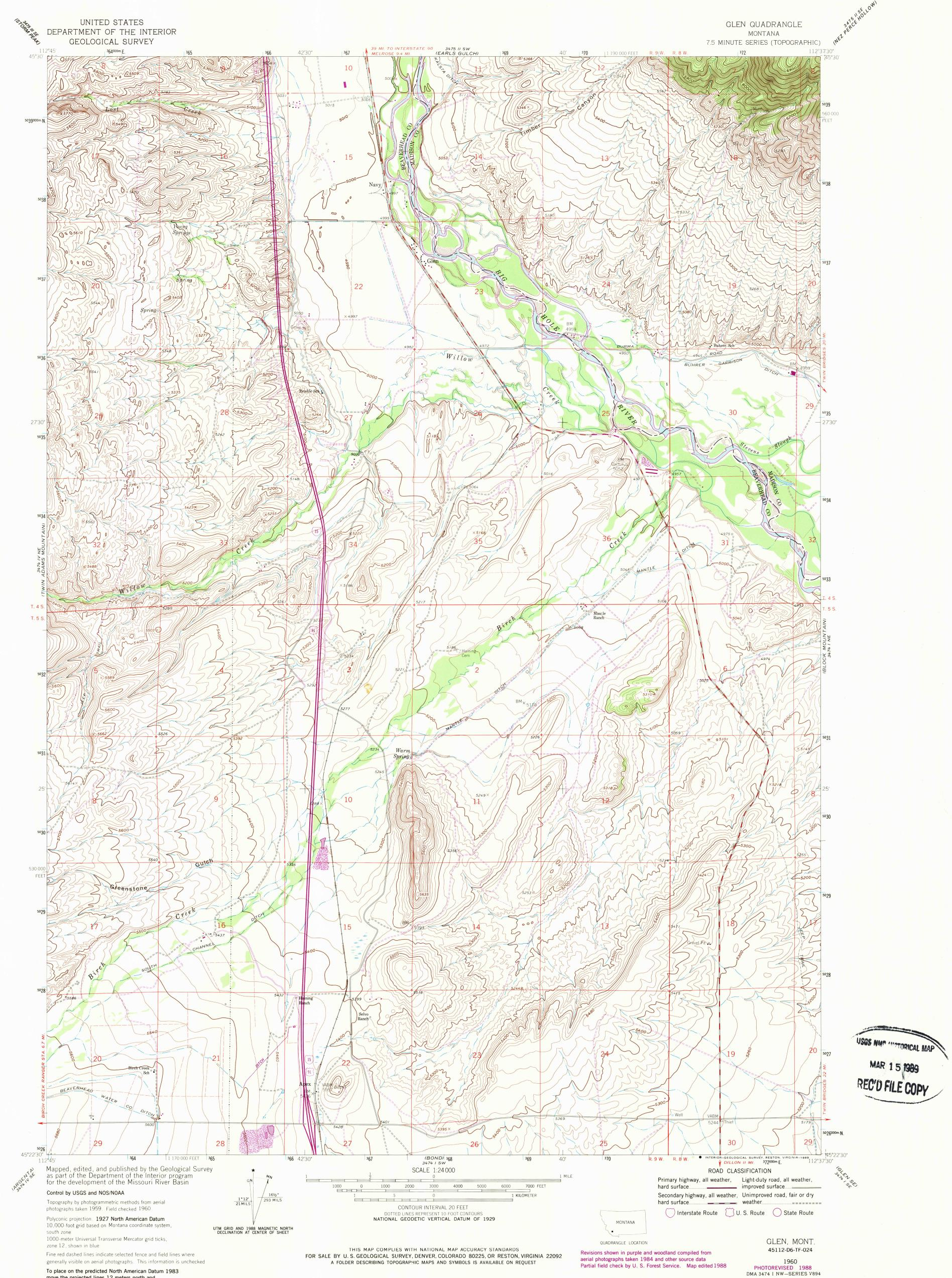
move the projected lines 12 meters north and 67 meters east as shown by dashed corner ticks
