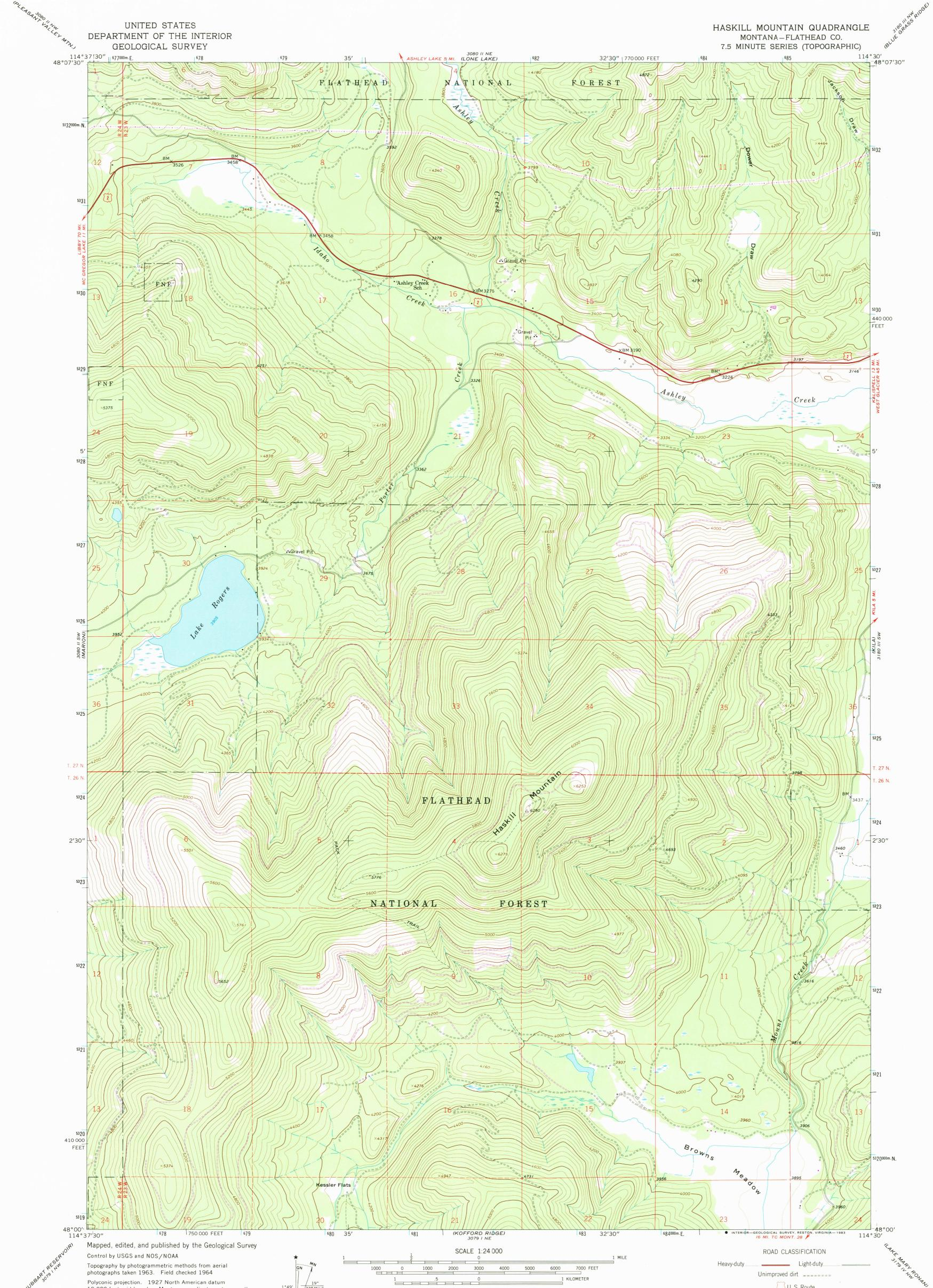
Polyconic projection. 1927 North American datum 1°49′ / 338 MILS 10,000-foot grid based on Montana coordinate system, north zone 1000-meter Universal Transverse Mercator grid ticks, zone 11, shown in blue
