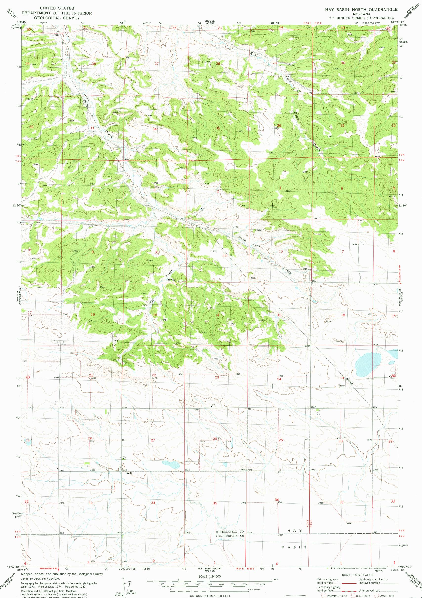
Projection and 10,000-foot grid ticks: Montana coordinate system, south zone (Lambert conformal conic) 1000-meter Universal Transverse Mercator grid, zone 12 1927 North American datum
