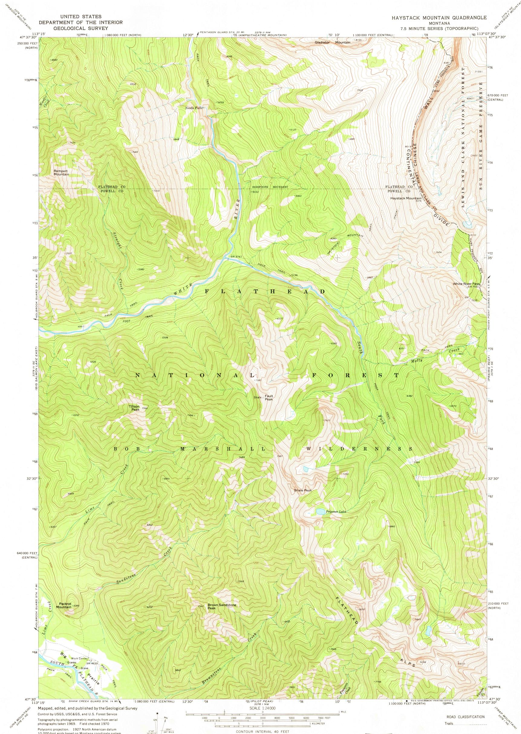
Polyconic projection. 1927 North American datum 10,000-foot grids based on Montana coordinate system, central and north zones 1000-meter Universal Transverse Mercator grid ticks, zone 12, shown in blue Land lines have not been established in this area
