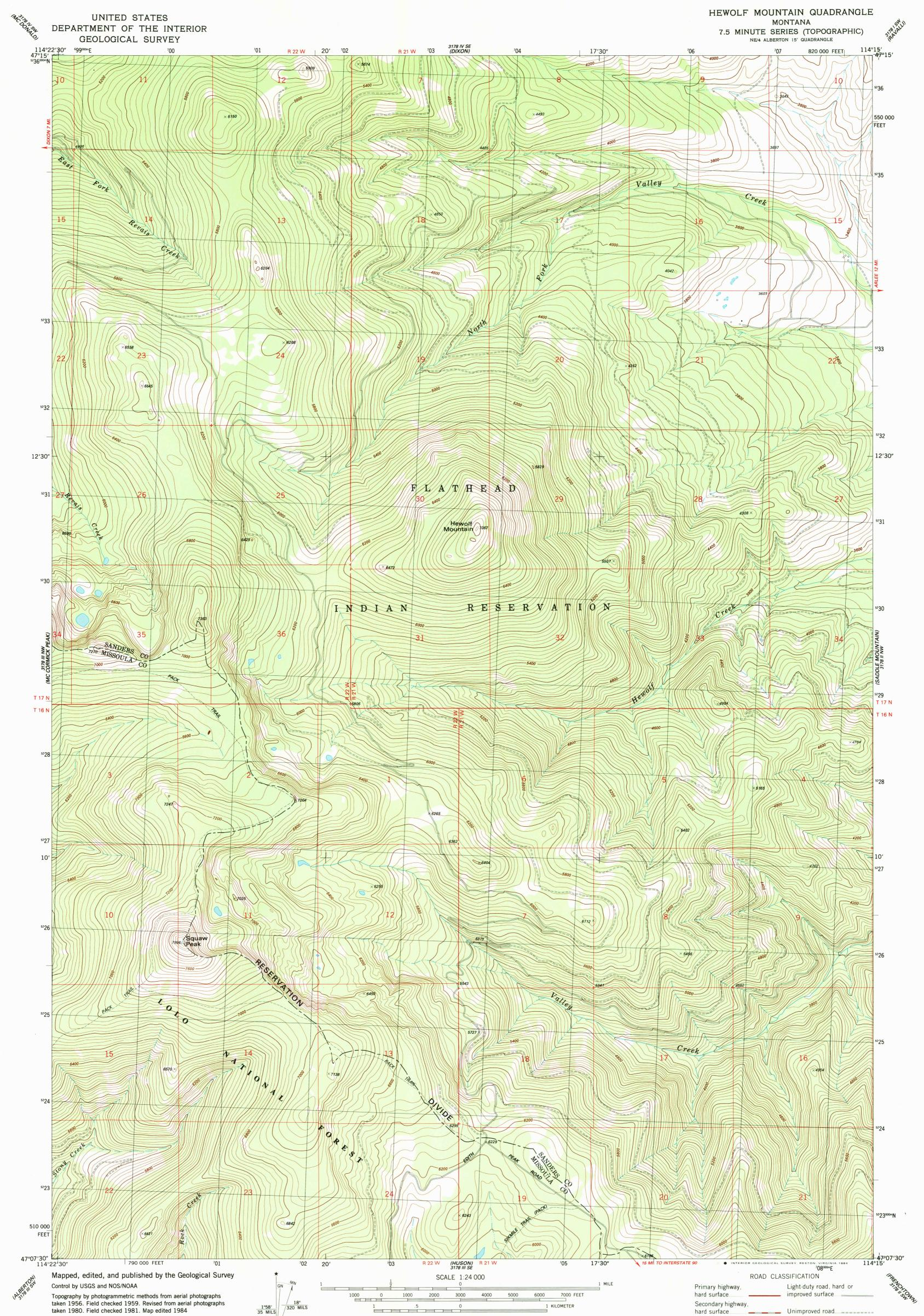
Projection and 10,000-foot grid ticks: Montana coordinate system, central zone (Lambert conformal conic) 1000-meter Universal Transverse Mercator grid, zone 11 1927 North American Datum To place on the predicted North American Datum 1983 move the projection lines 12 meters north and 71 meters east as shown by dashed corner ticks Fine red dashed lines indicate selected fence lines There may be private inholdings within the boundaries of
