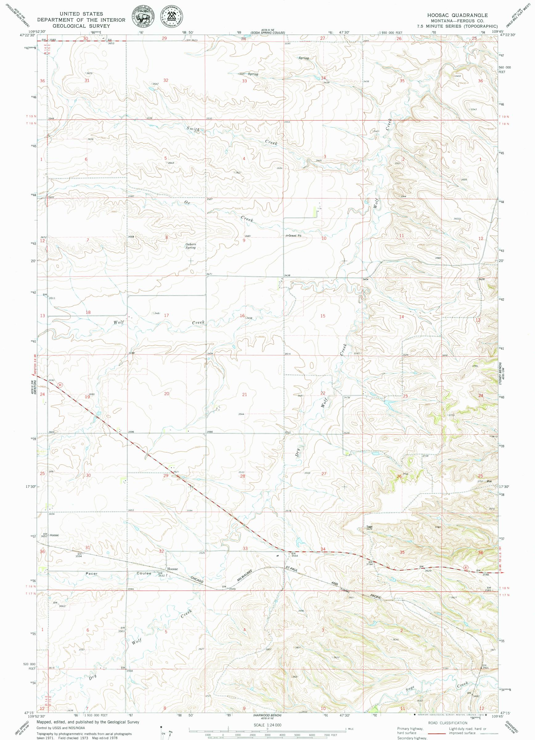
Projection and 10,000-foot grid ticks: Montana coordinate system, central zone (Lambert conformal conic) 1000-meter Universal Transverse Mercator grid ticks, zone 12, shown in blue. 1927 North American datum
