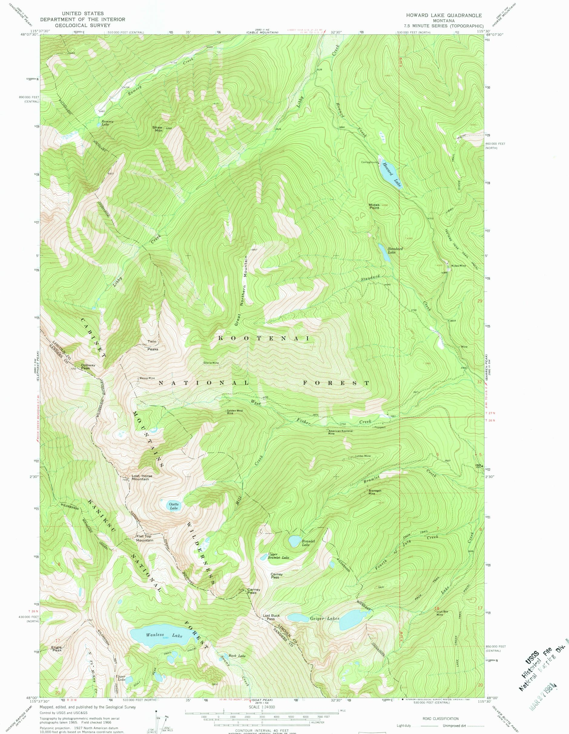
Polyconic projection. 1927 North American datum 10,000-foot grids based on Montana coordinate system, north and central zones 1000-meter Universal Transverse Mercator grid ticks, zone 11, shown in blue
