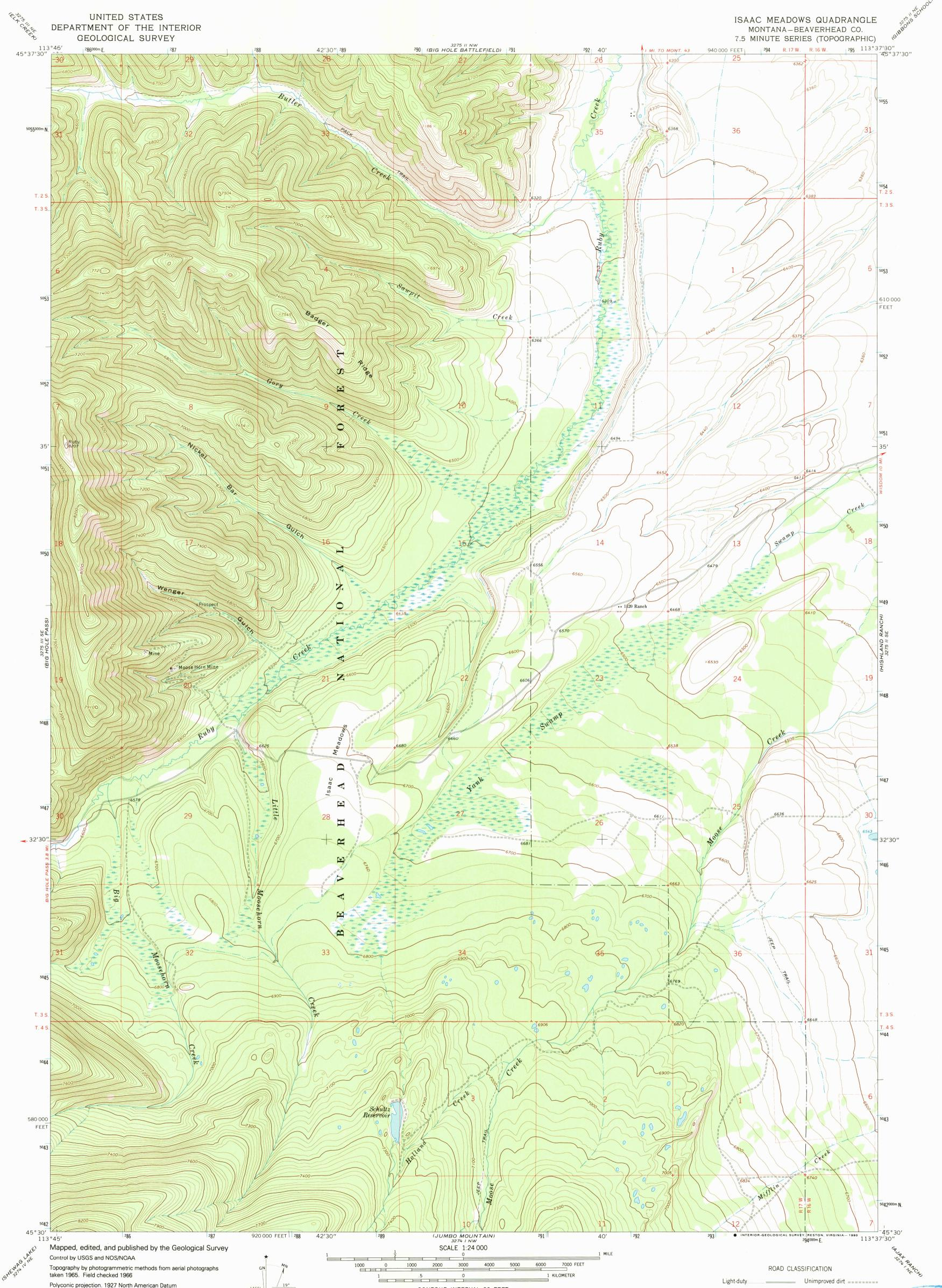
10,000-foot grid based on Montana coordinate system, south zone 1000-meter Universal Transverse Mercator grid ticks, zone 12 shown in blue To place on the predicted North American Datum 1983 move the projection lines 12 meters north and 70 meters east as shown by dashed corner ticks
