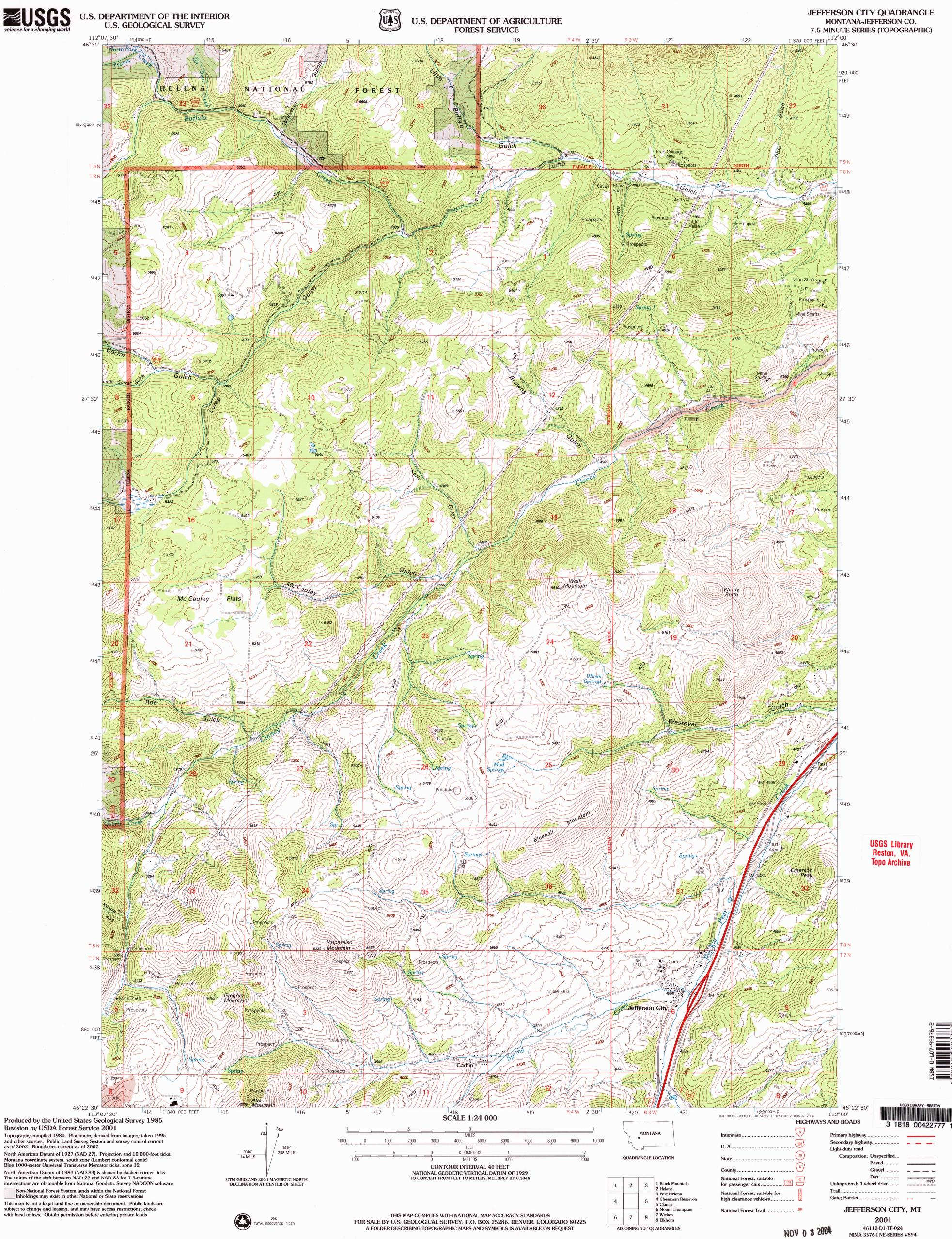
Montana coordinate system, south zone (Lambert conformal conic) Blue 1000-meter Universal Transverse Mercator ticks, zone 12 North American Datum of 1983 (NAD 83) is shown by dashed corner ticks The values of the shift between NAD 27 and NAD 83 for 7.5-minute intersections are obtainable from National Geodetic Survey NADCON software Inholdings may exist in other National or State reservations This map is not a legal land line or ownership document. Public lands are
