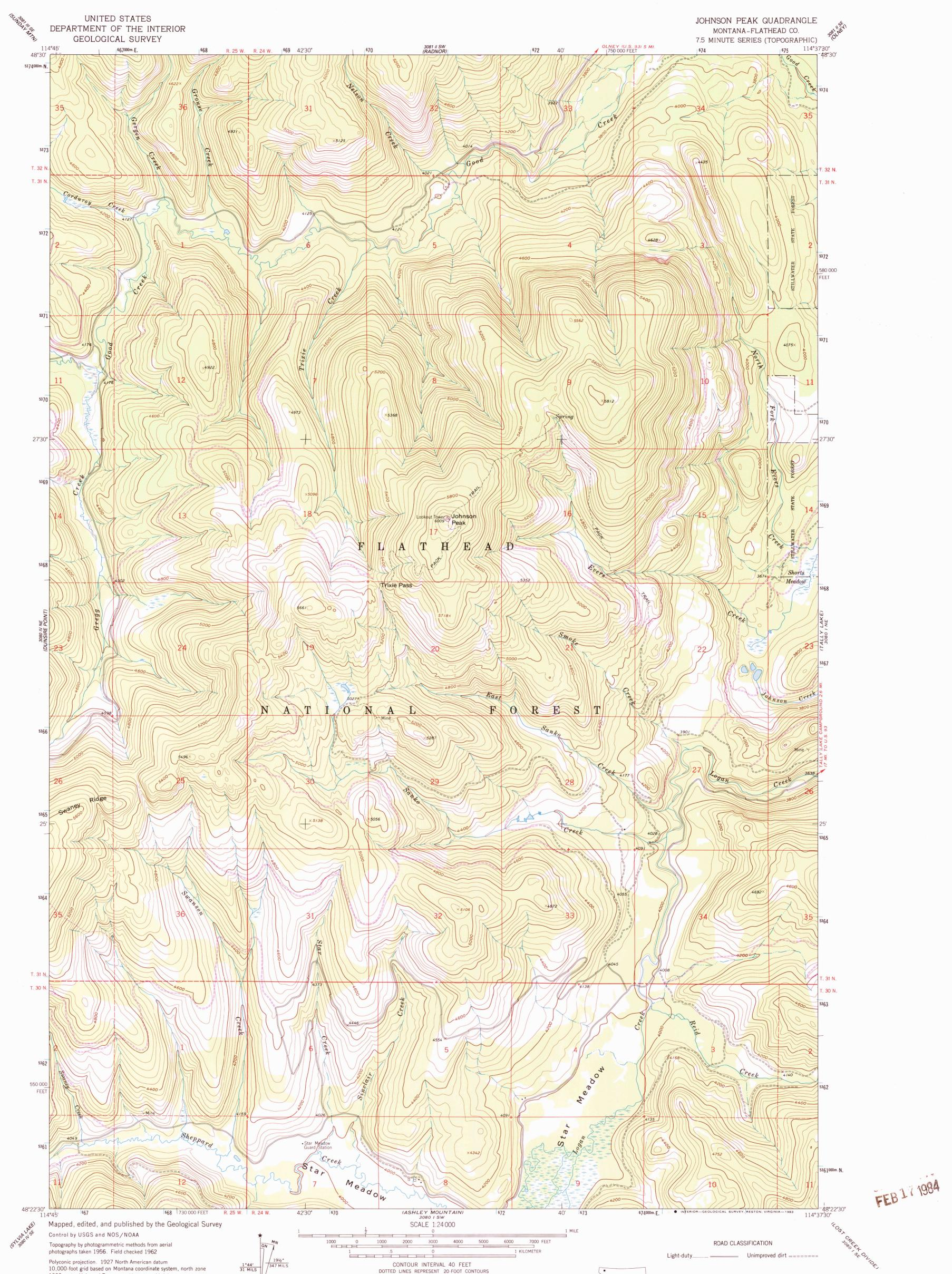
Polyconic projection. 1927 North American datum 10,000-foot grid based on Montana coordinate system, north zone 1000-meter Universal Transverse Mercator grid ticks, zone 11, shown in blue
