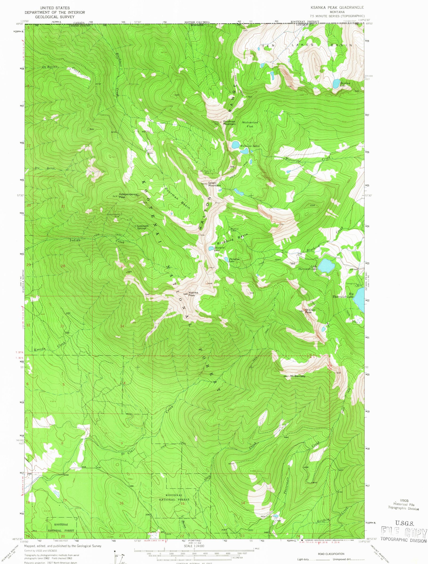
Polyconic projection. 1927 North American datum 10,000-foot grid bašed on Montana coordinate system, north zone 1000-meter Universal Transverse Mercator grid ticks, zone 11, shown in blue
