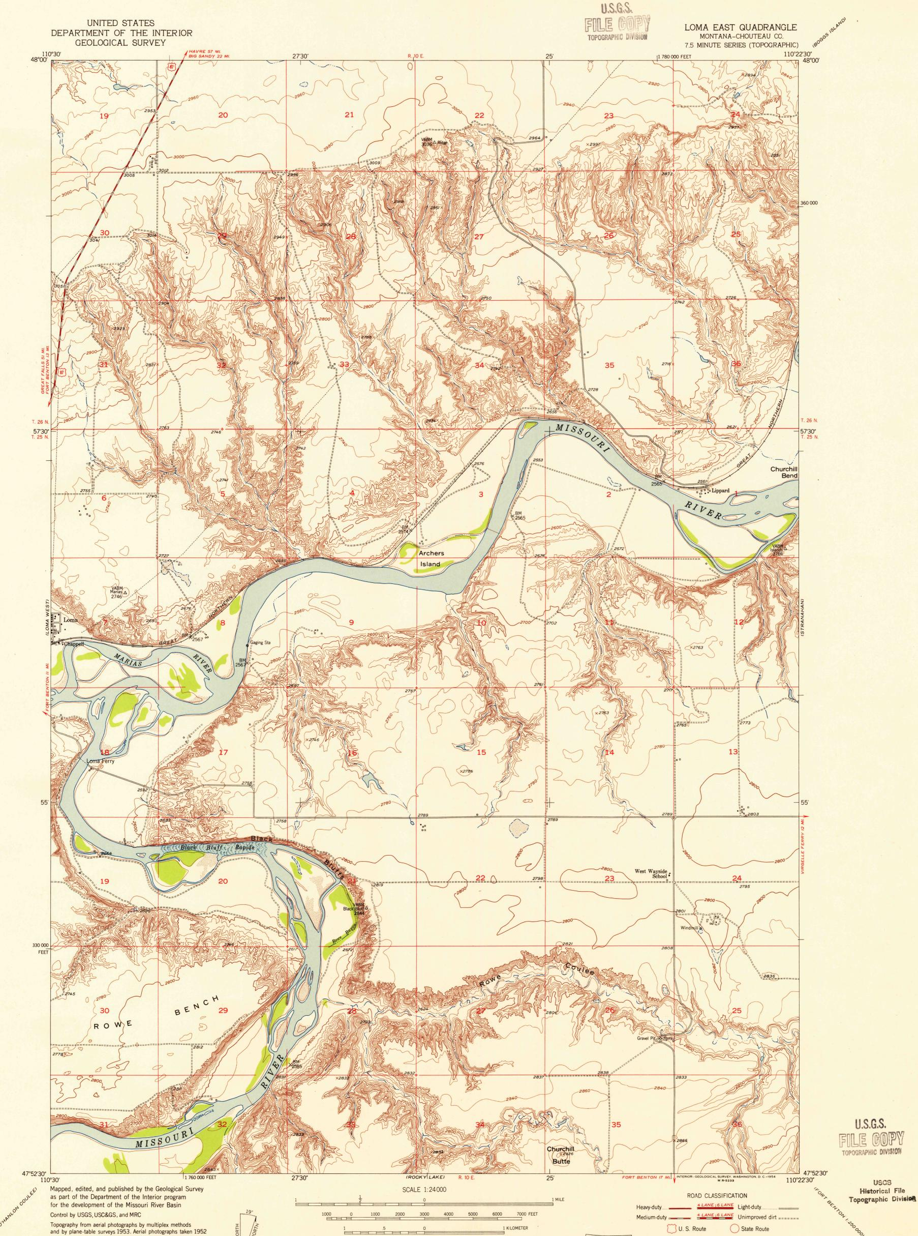
Topography from aerial photographs by multiplex methods and by plane-table surveys 1953. Aerial photographs taken 1952 Polyconic projection. 1927 North American datum 10,000-foot grid based on Montana coordinate system, north zone
