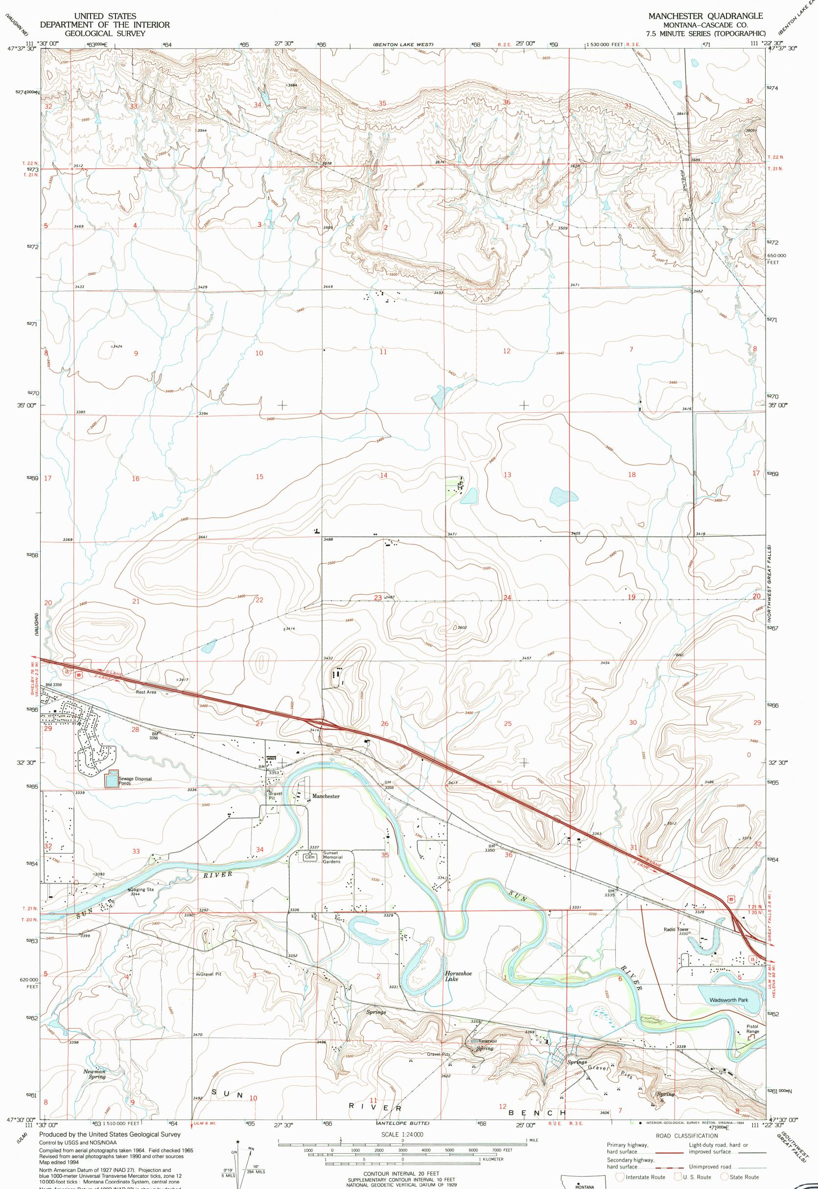
blue 1000-meter Universal Transverse Mercator ticks, zone 12 6 MILS 10000-foot ticks : Montana Coordinate System, central zone North American Datum of 1983 (NAD 83) is shown by dashed corner ticks. The values of the shift between NAD 27 and NAD 83 for 7.5-minute intersections are obtainable from National Geodetic Support NADCON software Survey NADCON software
