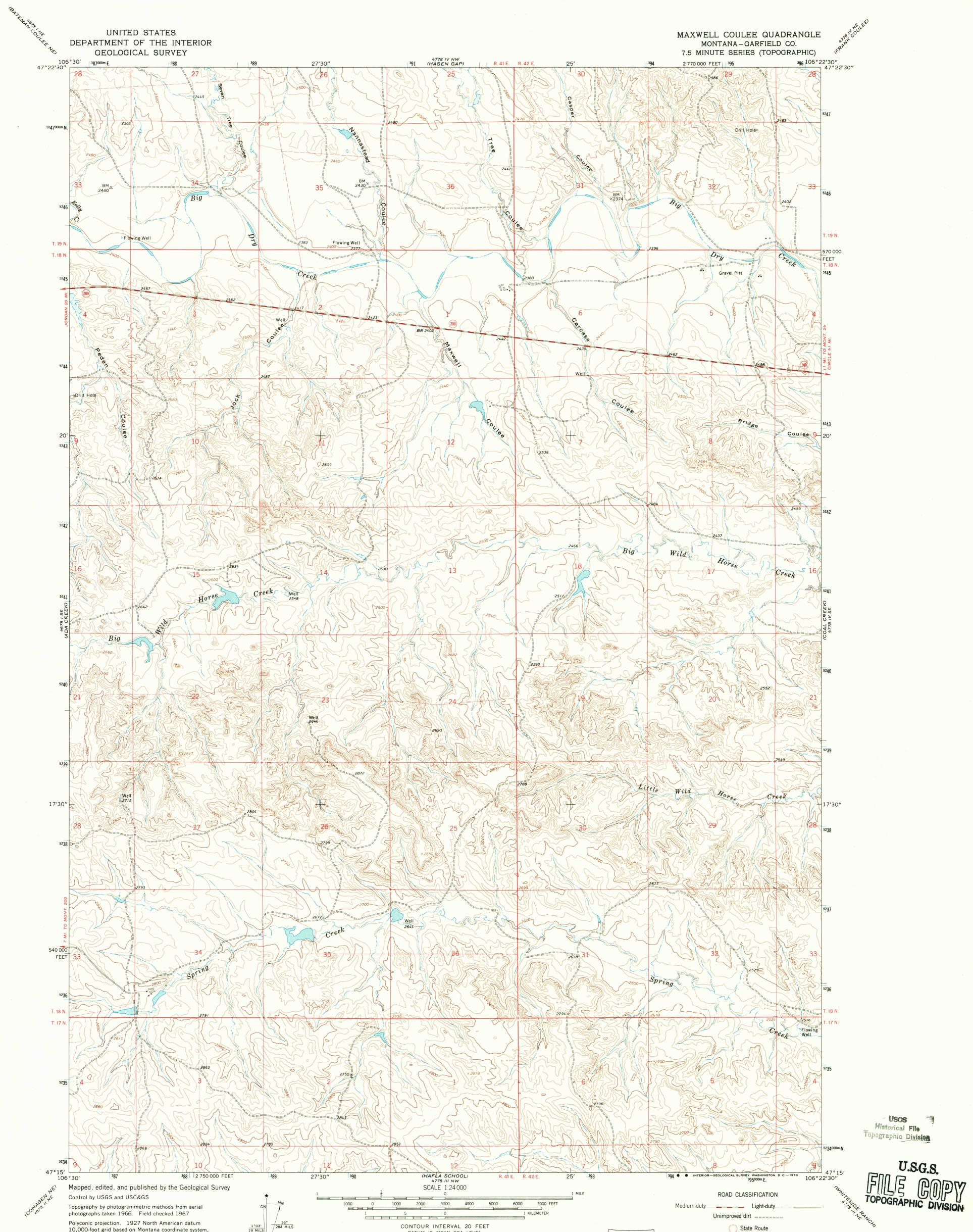
(0° k° photographs taken 1966. Field checked 1967 Polyconic projection. 1927 North American datum 10,000-foot grid based on Montana coordinate system, 1°03' 19 MILS central zone 1000-meter Universal Transverse Mercator grid ticks, zone 13, shown in blue UTM GRID AND 1967 MAGNETIC NORTH DECLINATION AT CENTER OF SHEET
