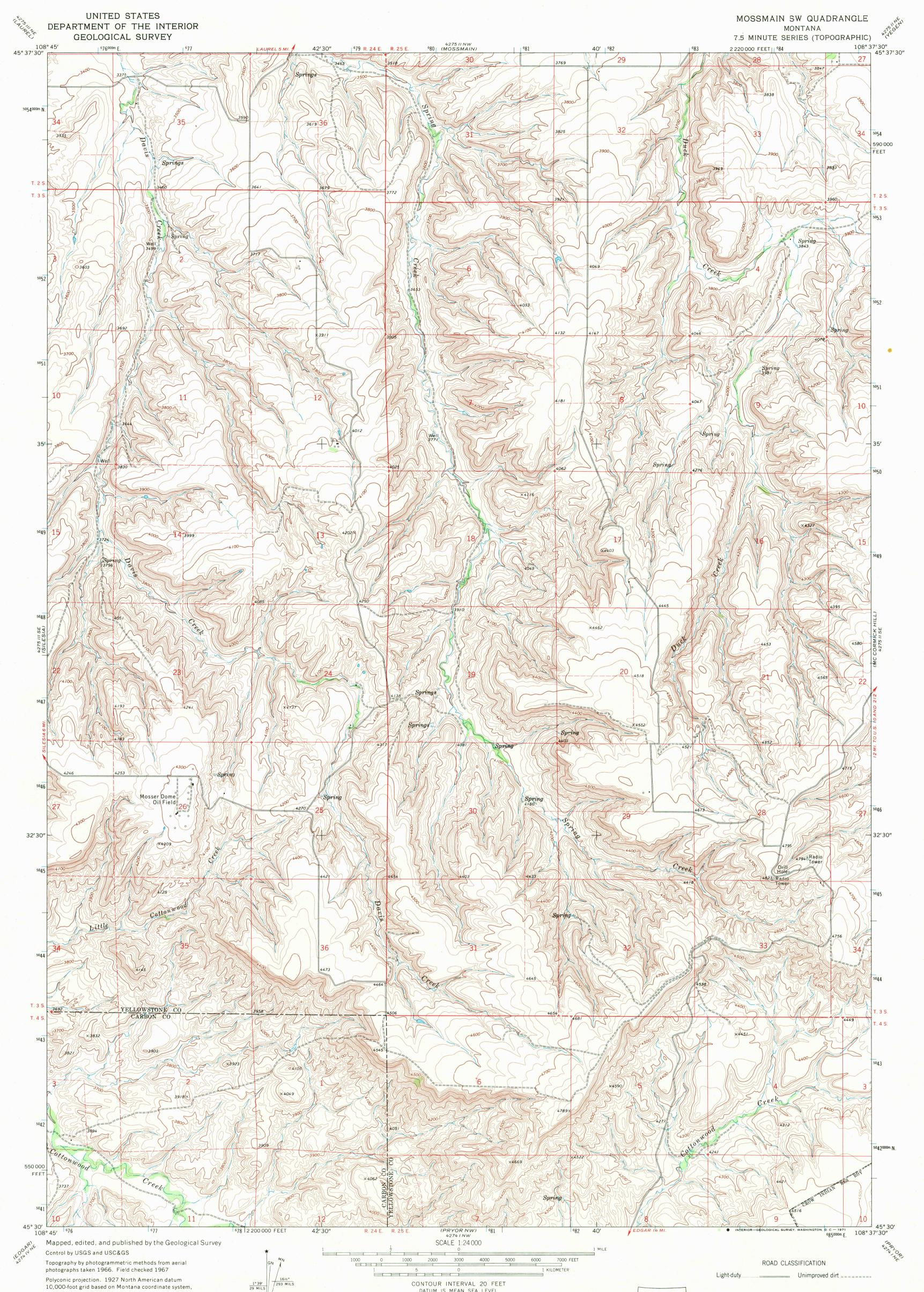
10,000-foot grid based on Montana coordinate system, south zone 1000-meter Universal Transverse Mercator grid ticks, zone 12, shown in blue Fine red dashed lines indicate selected fence lines
