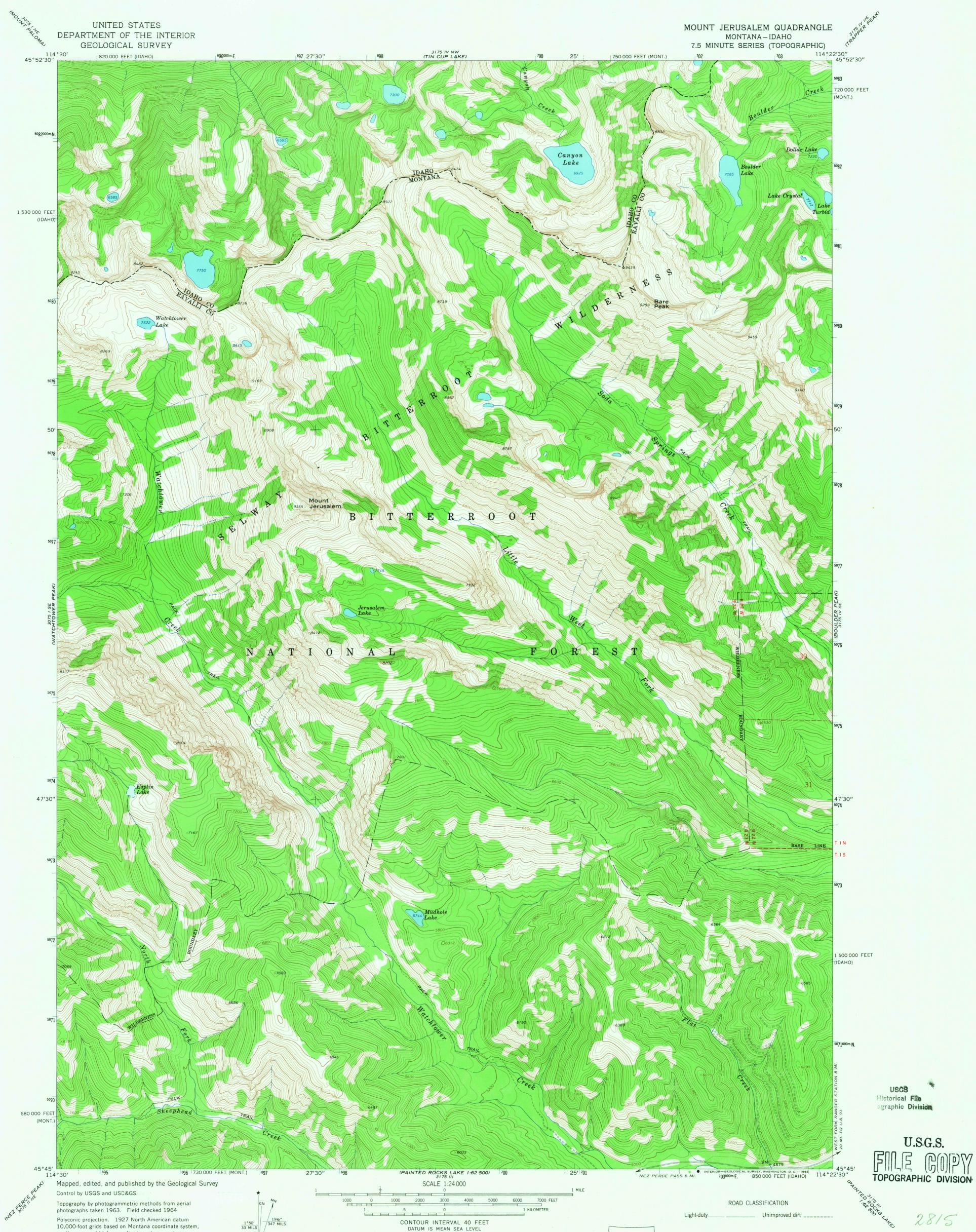
Polyconic projection. 1927 North American datum 10,000-foot grids based on Montana coordinate system, south zone, and Idaho coordinate system, west zone 1000-meter Universal Transverse Mercator grid ticks, zone 11, shown in blue
