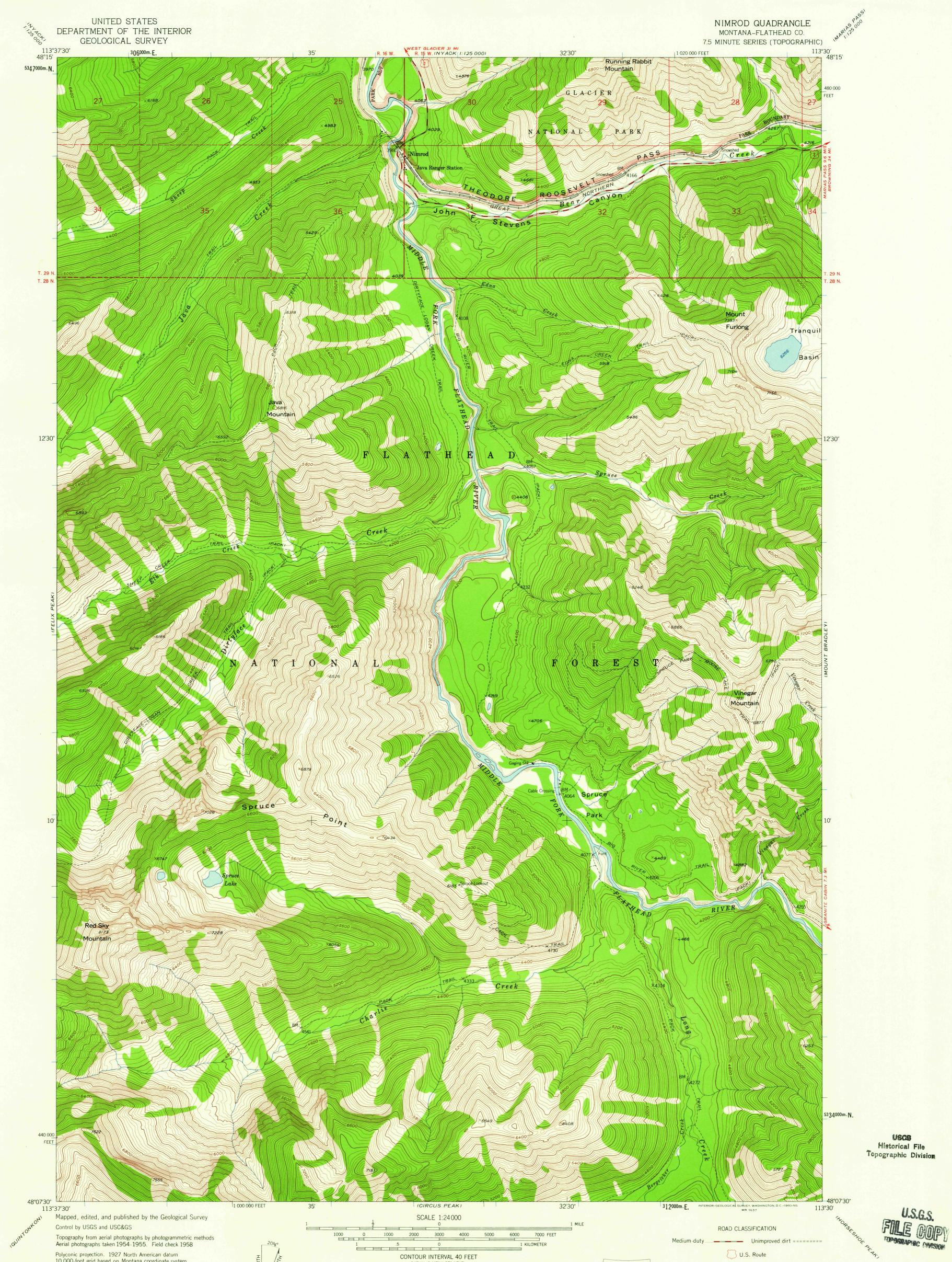
Polyconic projection. 1927 North American datum 10,000-foot grid based on Montana coordinate system, north zone 1000-meter Universal Transverse Mercator grid ticks, zone 12, shown in blue Dashed land lines indicate approximate locations Land lines unsurveyed except in T. 29 N.-Rs. 15 and 16 W.
