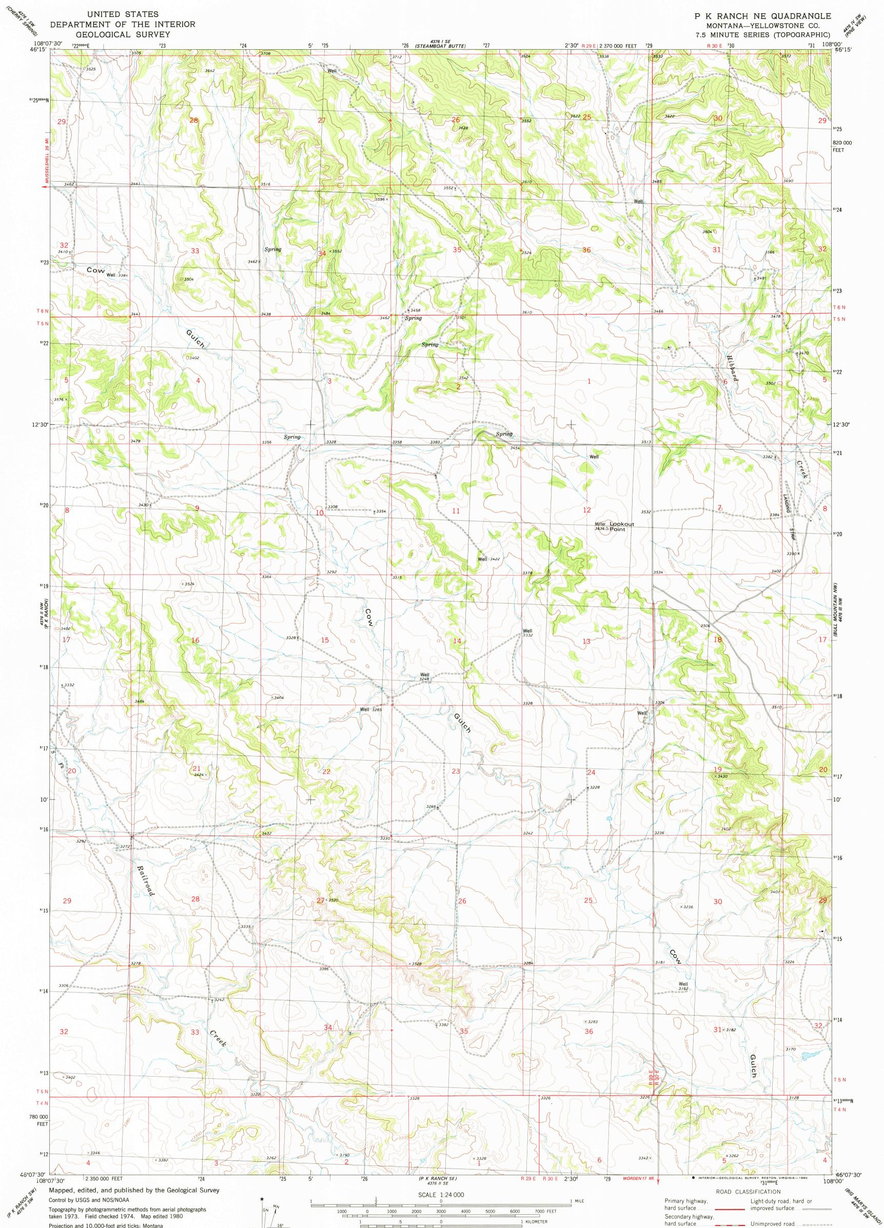
Projection and 10,000-foot grid ticks: Montana coordinate system, south zone (Lambert conformal conic) 1000-meter Universal Transverse Mercator grid, zone 12 1927 North American datum To place on the predicted North American Datum 1983 move the projection lines 8 meters north and
