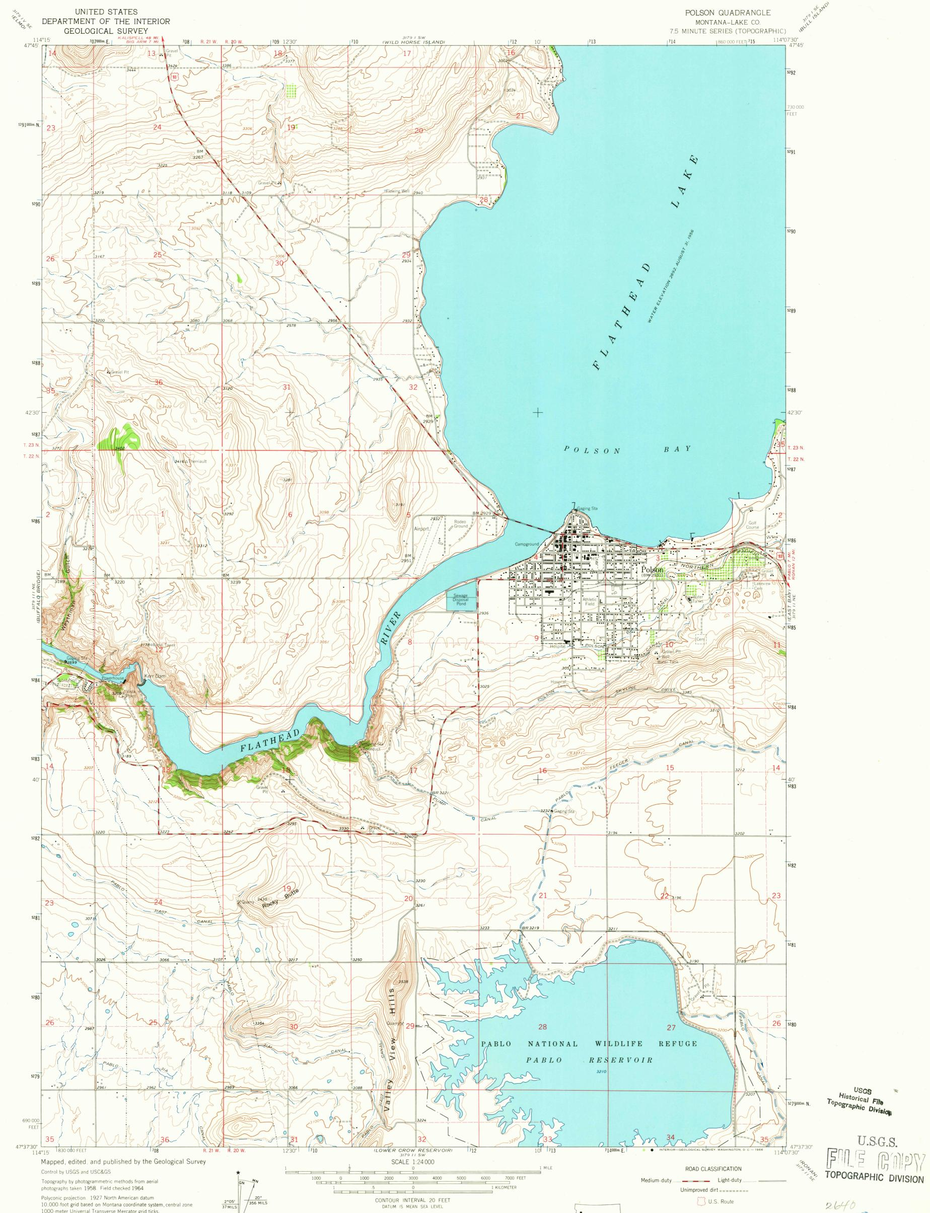
10,000-foot grid based on Montana coordinate system, central zone 1000 meter Universal Transverse Mercator grid ticks, zone 11, shown in blue
