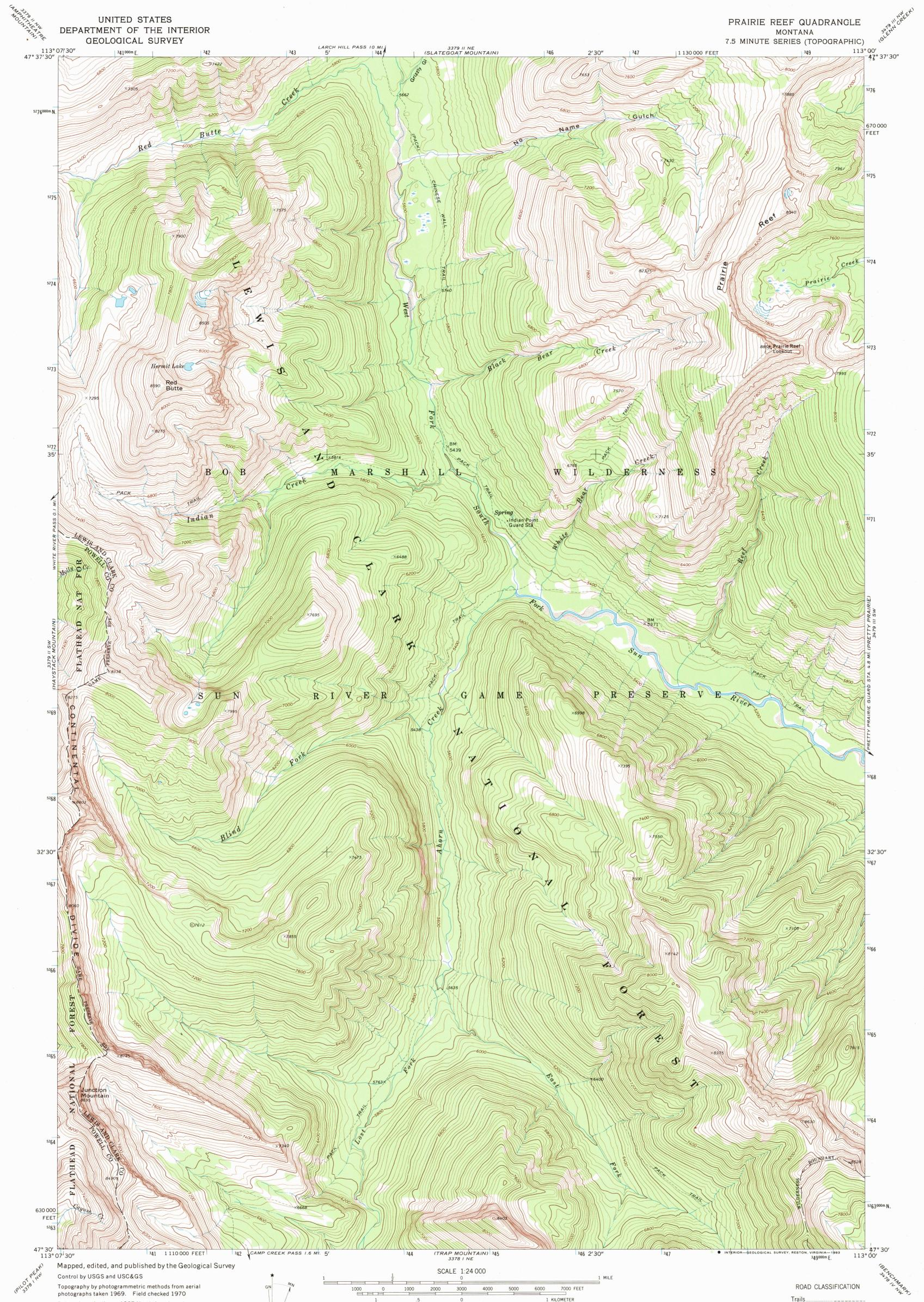
Polyconic projection. 1927 North American datum 10,000-foot grid based on Montana coordinate system, central zone 1000-meter Universal Transverse Mercator grid ticks, zone 12, shown in blue Land lines have not been established in this area To place on the predicted North American Datum 1983 move the projection lines 10 meters north and 67 meters east as shown by dashed corner ticks There may be private inholdings within the boundaries of the
