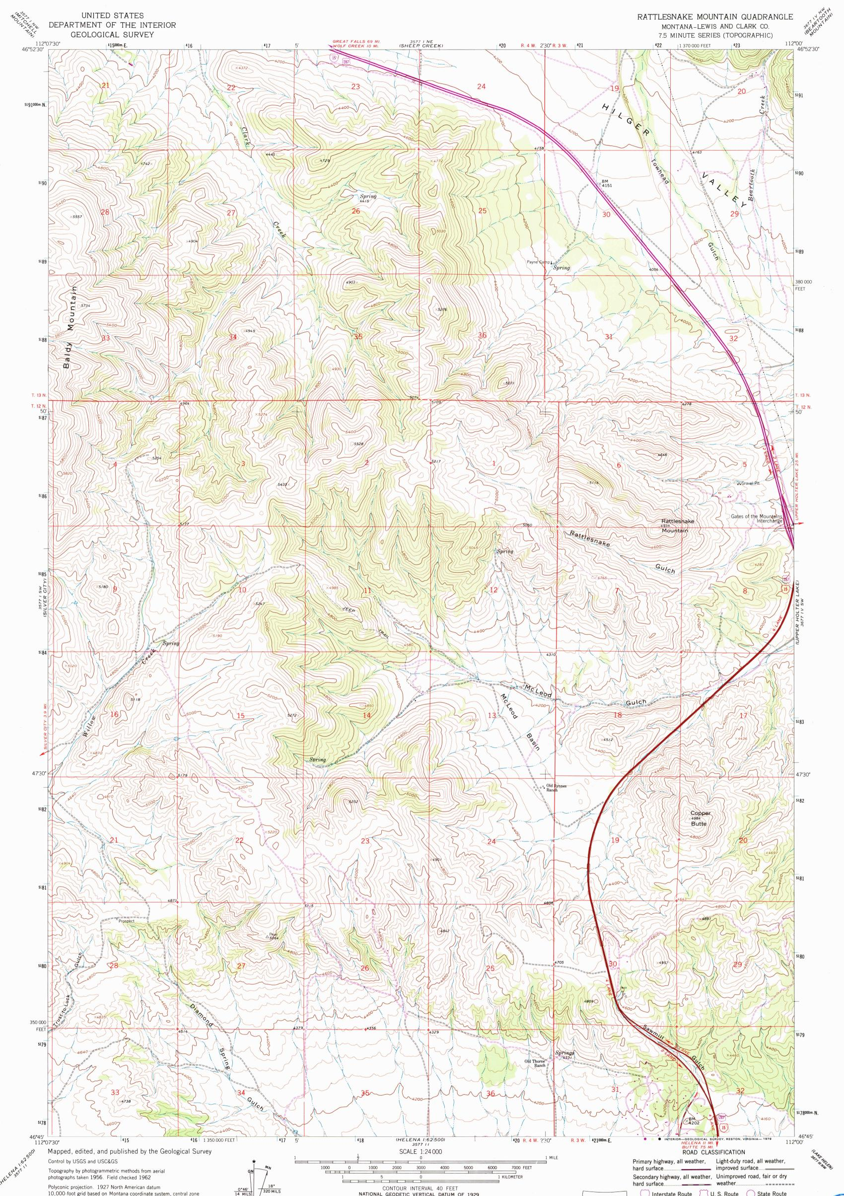
Polyconic projection. 1927 North American datum 10,000-foot grid based on Montana coordinate system, central zone 1000-meter Universal Transverse Mercator grid ticks, zone 12, shown in blue
