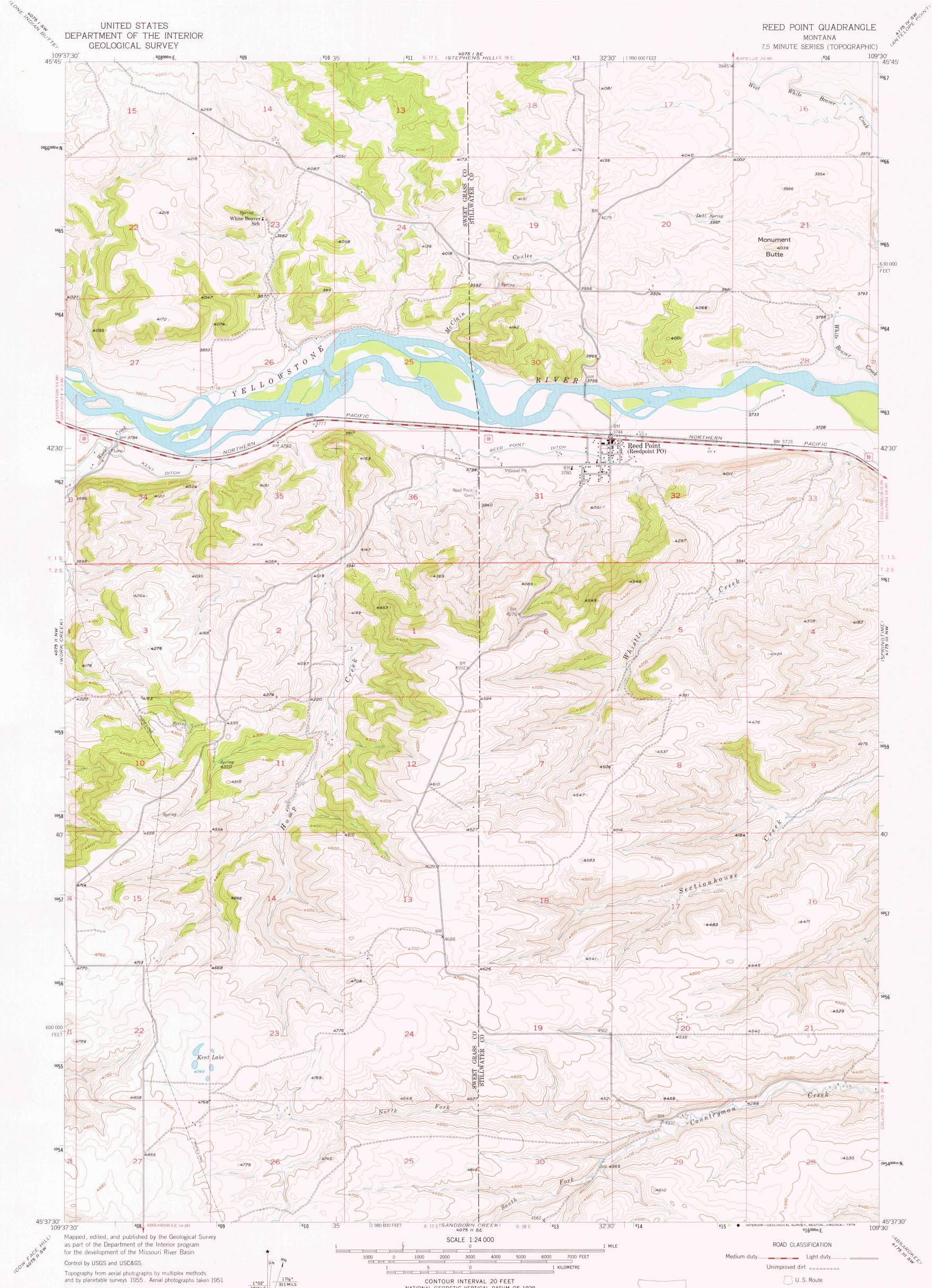
and by planetable surveys 1955. Aerial photographs taken 1951 Polyconic projection. 1927 North American datum 10,000-foot grid based on Montana coordinate system, south zone 1000-metre Universal Transverse Mercator grid ticks, UTM GRID AND 1955 MAGNETIC NORTH DECLINATION AT CENTER OF SHEET zone 12, shown in blue
