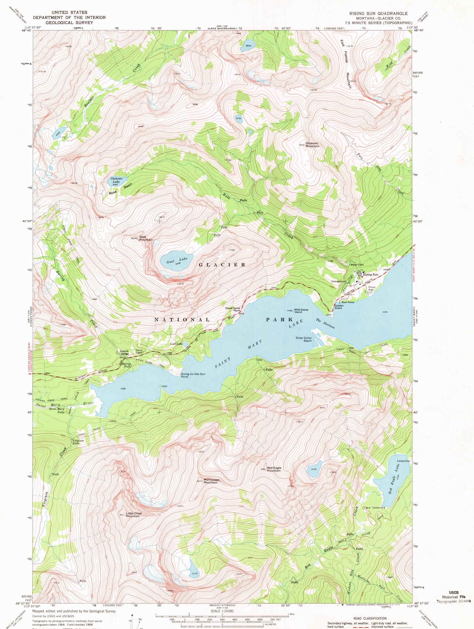
Polyconic projection. 1927 North American datum 10,000-foot grid based on Montana coordinate system, north zone 1000-meter Universal Transverse Mercator grid ticks, zone 12, shown in blue Land lines have not been established in this area UTM GRID AND 1968 MAGNETIC NORTH DECLINATION AT CENTER OF SHEET
