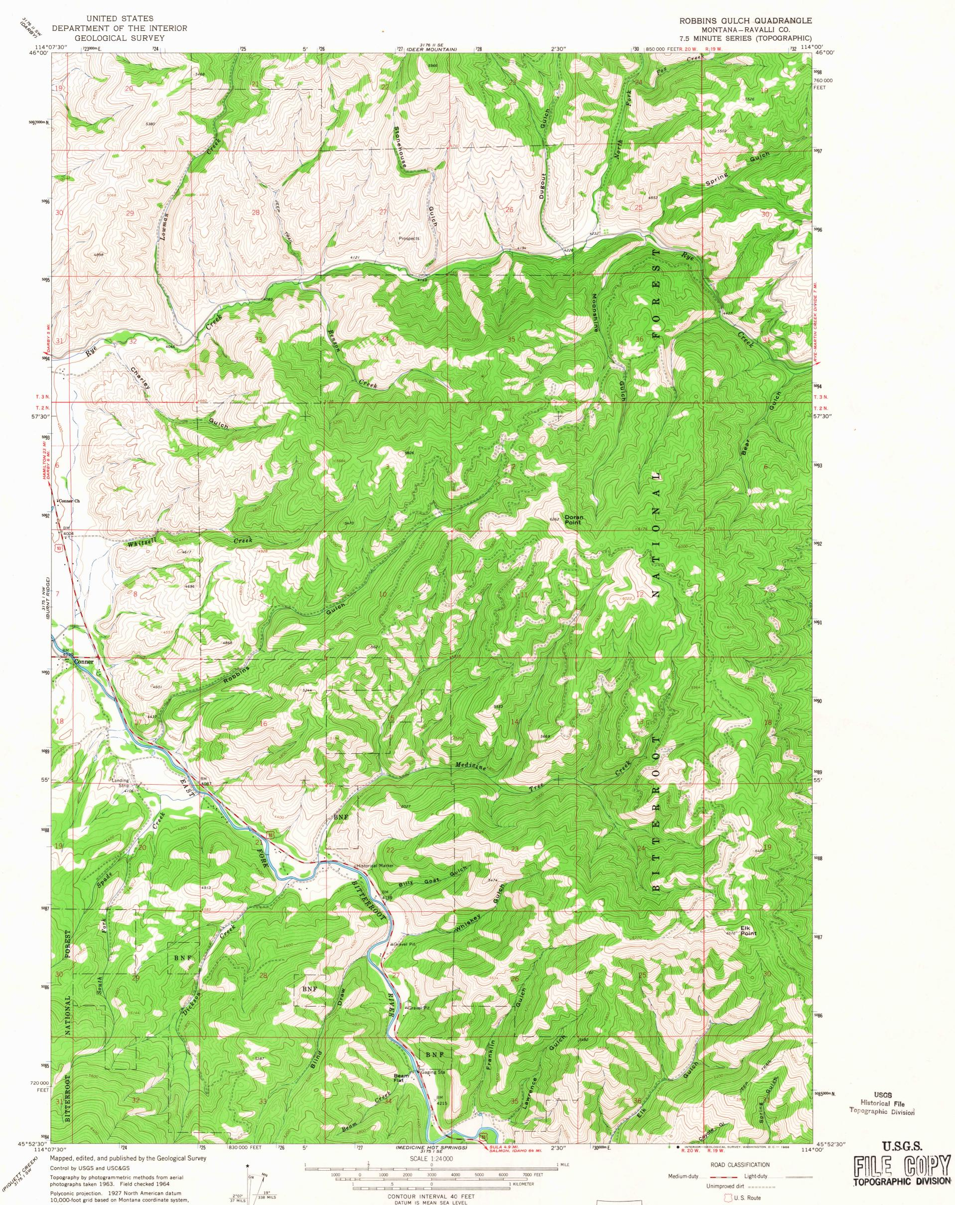
Polyconic projection. 1927 North American datum 10,000-foot grid based on Montana coordinate system, south zone 1000-meter Universal Transverse Mercator grid ticks, zone 11, shown in blue UTM GRID AND 1964 MAGNETIC NORTH DECLINATION AT CENTER OF SHEET Fine red dashed lines indicate selected fence lines
