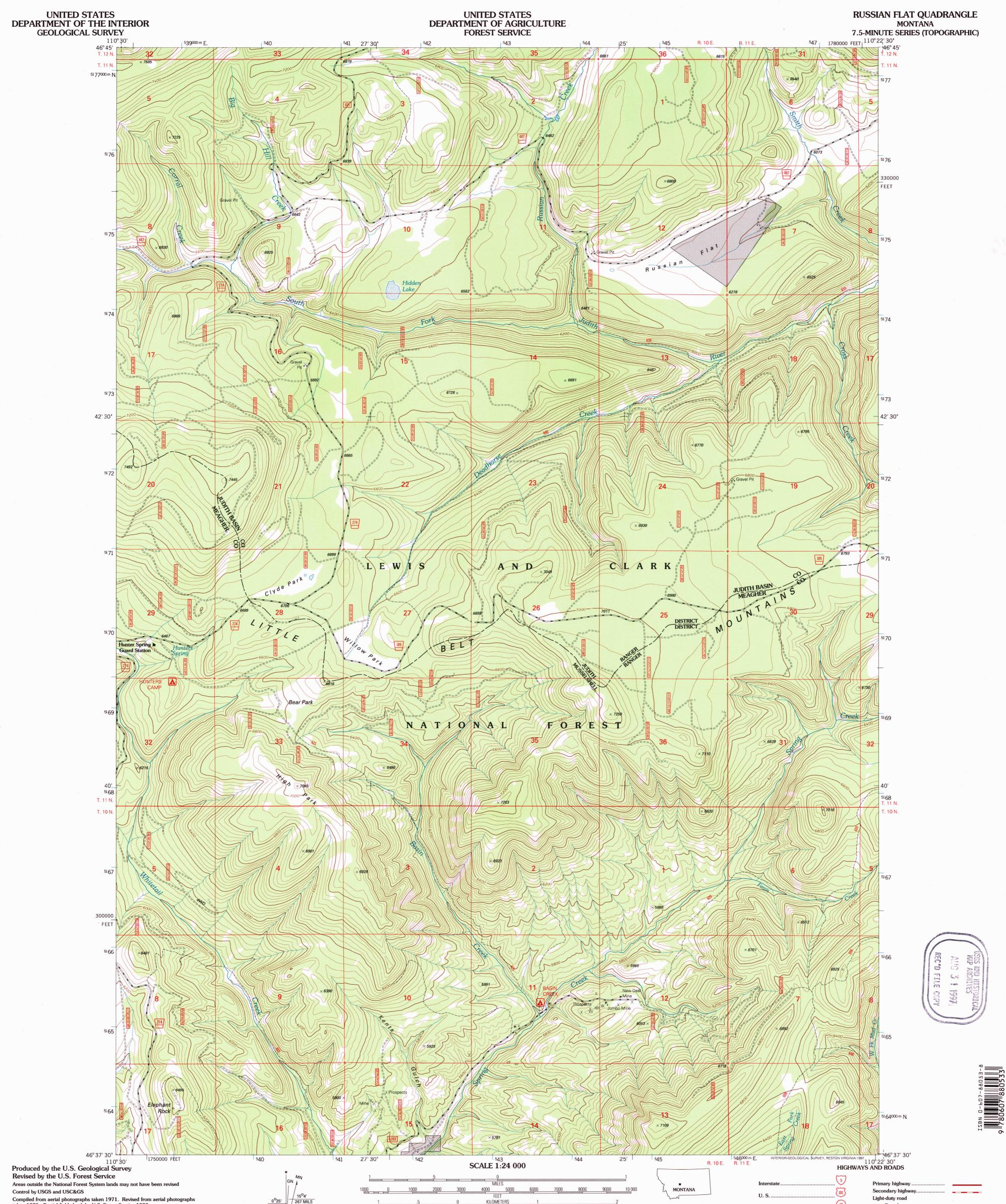
taken 1995. Partial field check by U.S. Forest Service 1995 North American Datum of 1927 (NAD 27). Projection and 10 000-foot ticks: Montana coordinate system, central zone (Lambert conformal conic). Blue 1000-meter Universal Transverse Mercator ticks, zone 12
