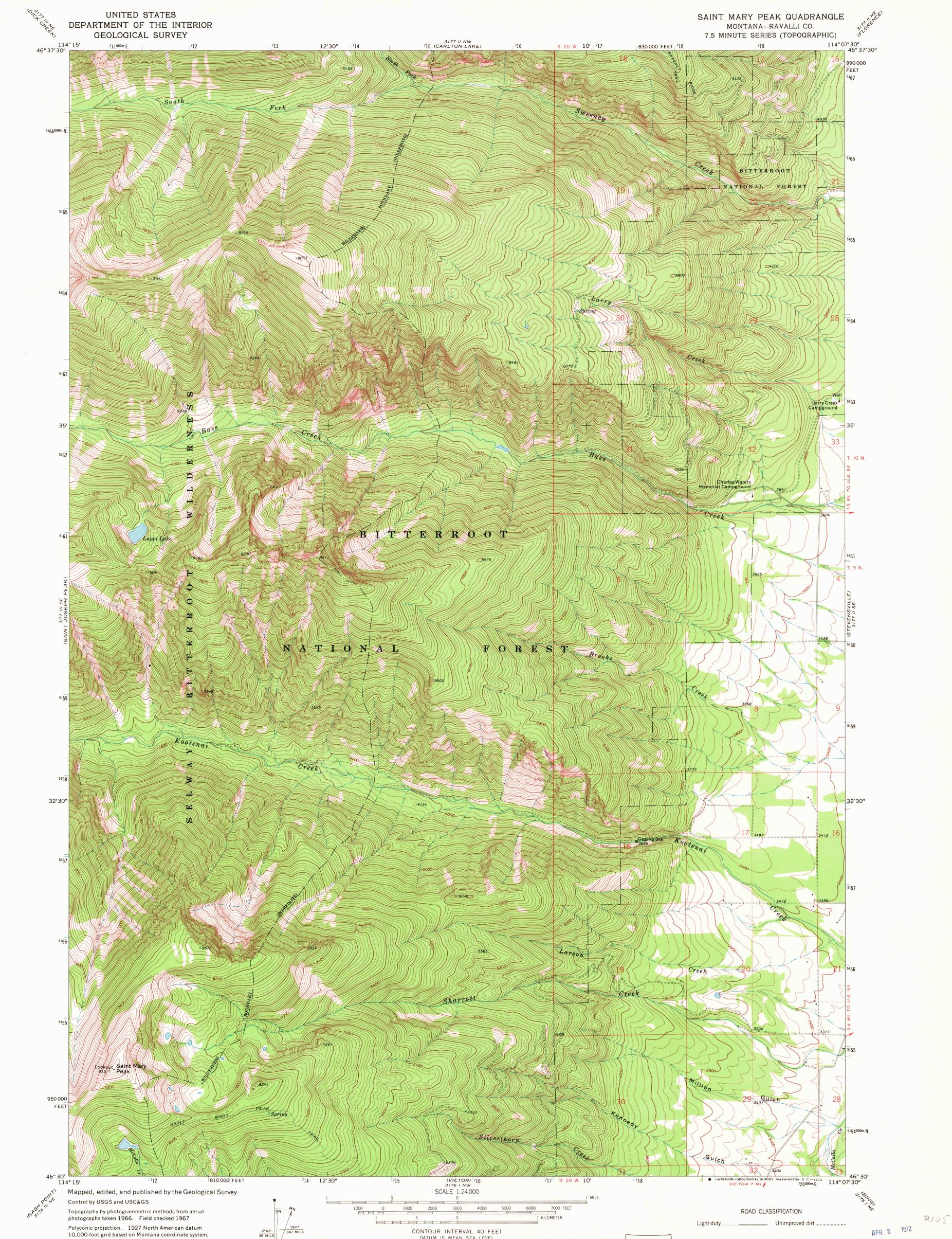
10,000-foot grid based on Montana coordinate system, south zone 1000-meter Universal Transverse Mercator grid ticks, zone 11, shown in blue Fine red dashed lines indicate selected fence lines
