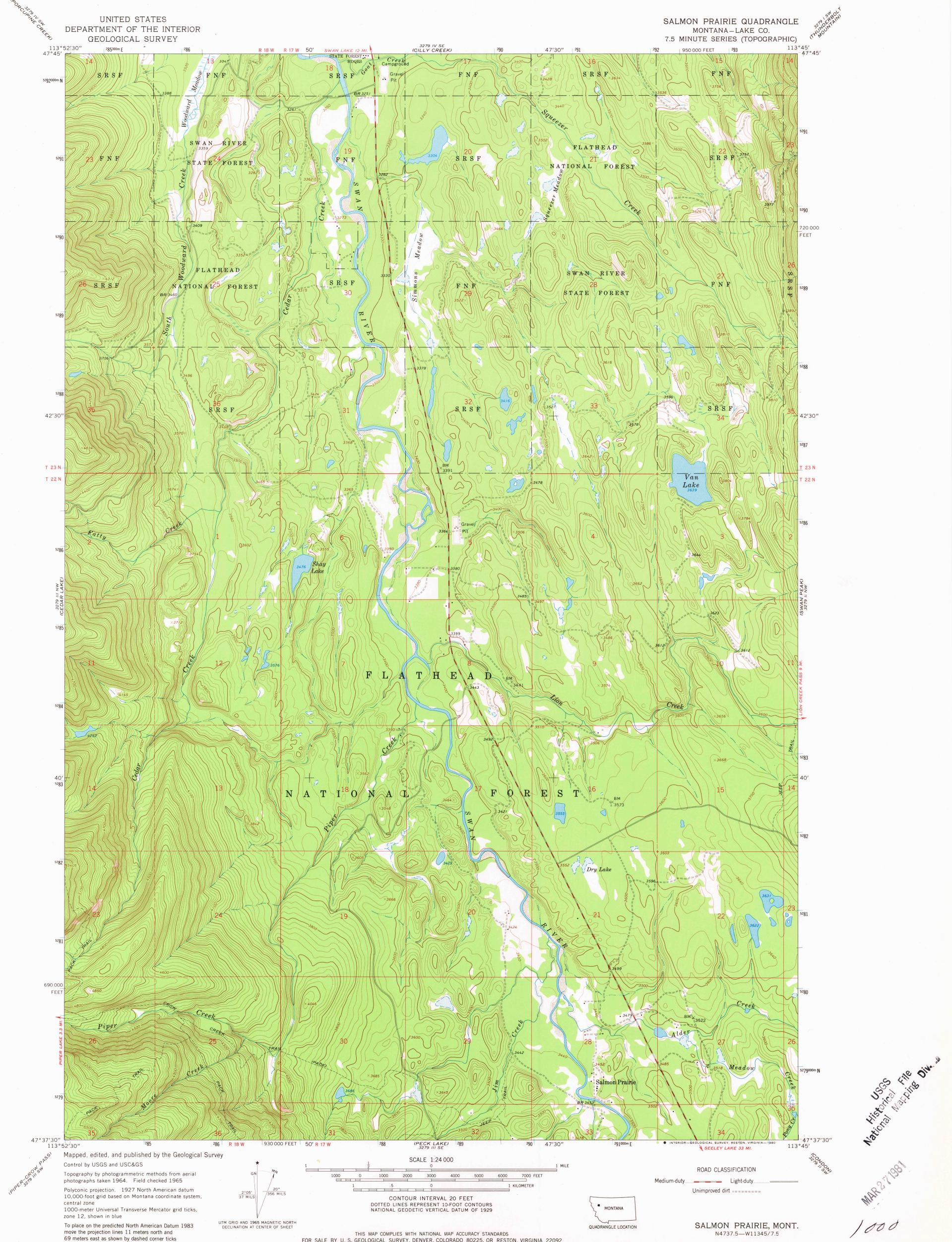
Polyconic projection. 1927 North American datum 10,000-foot grid based on Montana coordinate system, central zone 1000-meter Universal Transverse Mercator grid ticks, zone 12, shown in blue To place on the predicted North American Datum 1983 move the projection lines 11 meters north and 69 meters east as shown by dashed corner ticks
