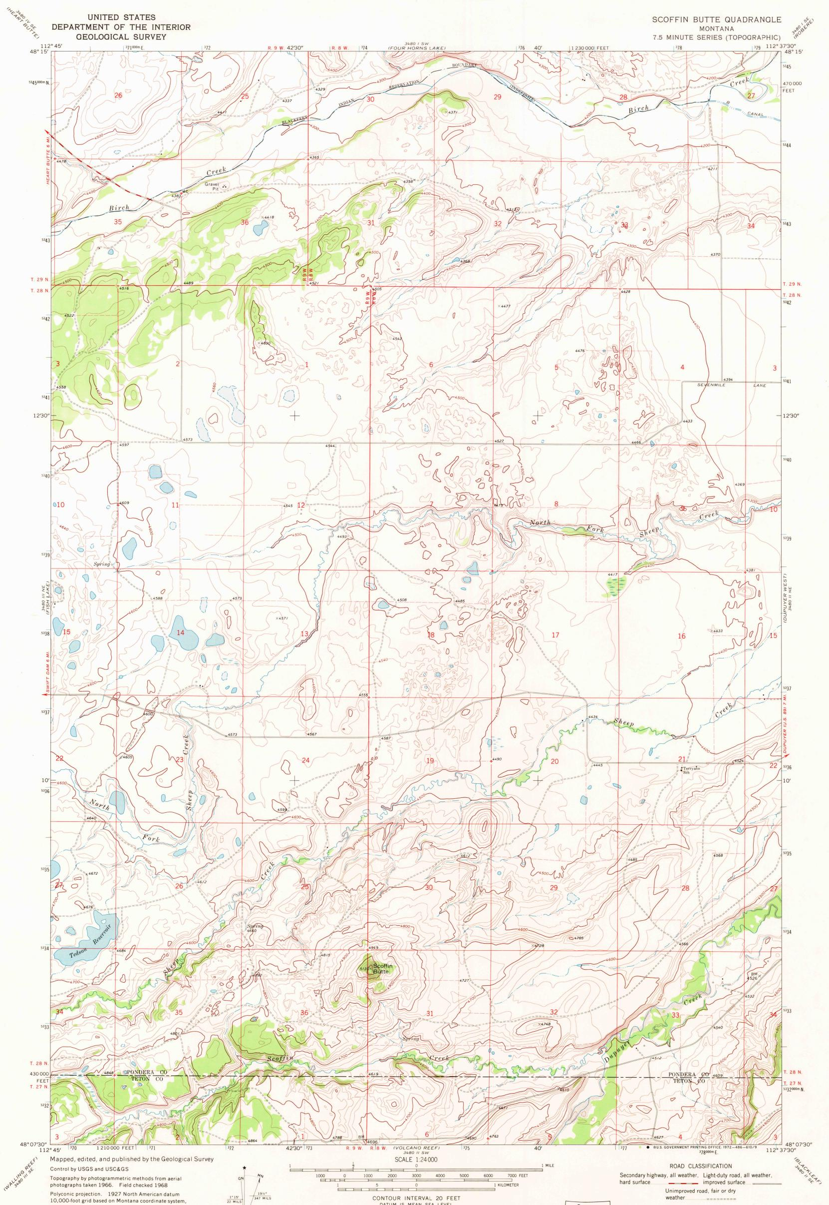
Polyconic projection. 1927 North American datum 10,000-foot grid based on Montana coordinate system, north zone 1000-meter Universal Transverse Mercator grid ticks, zone 12, shown in blue UTM GRID AND 1968 MAGNETIC NORTH DECLINATION AT CENTER OF SHEET Fine red dashed lines indicate selected fence lines
