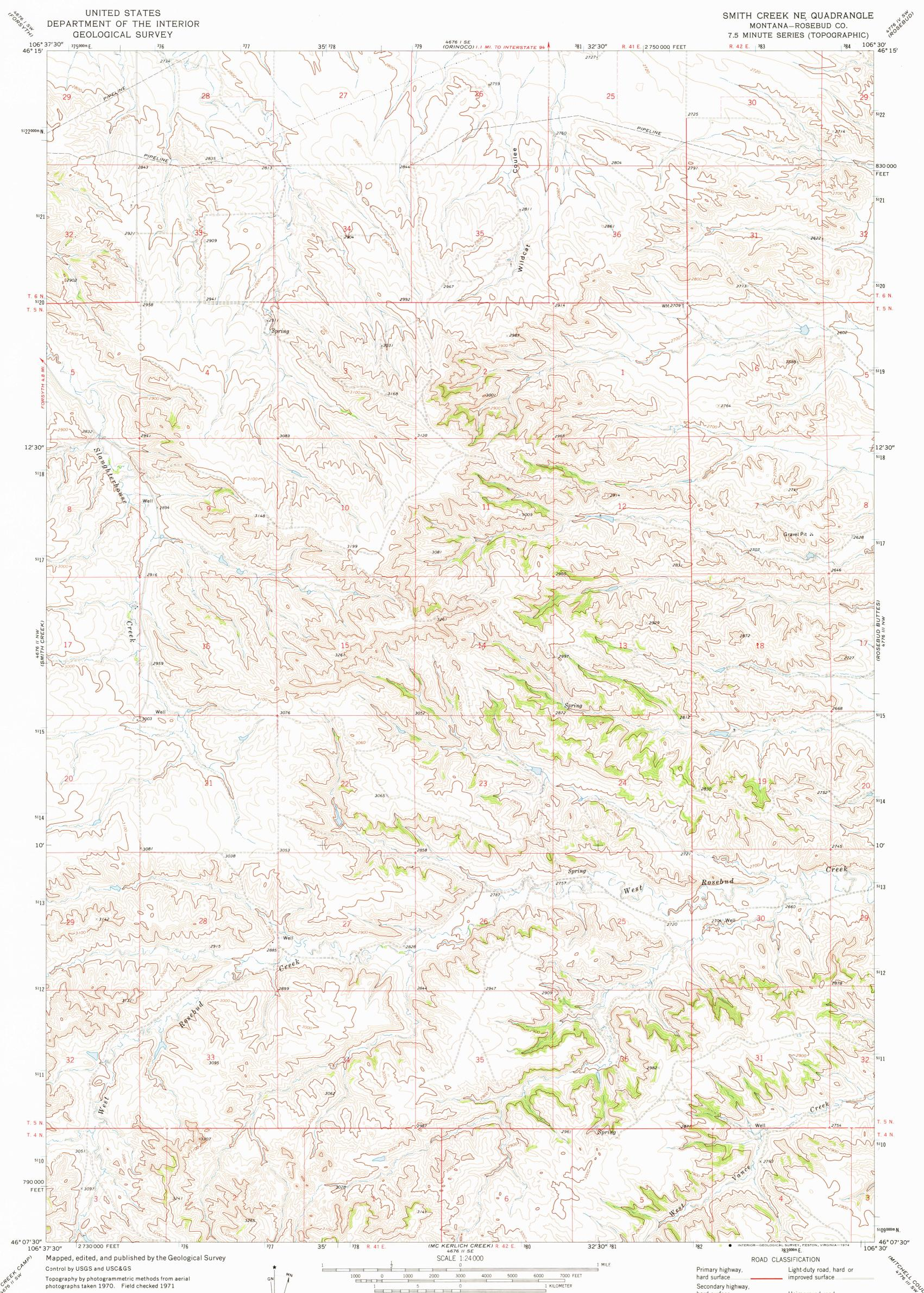
Projection and 10,000-foot grid ticks: Montana coordinate system, south zone (Lambert conformal conic) 1000-meter Universal Transverse Mercator grid ticks, zone 13, shown in blue. 1927 North American datum
