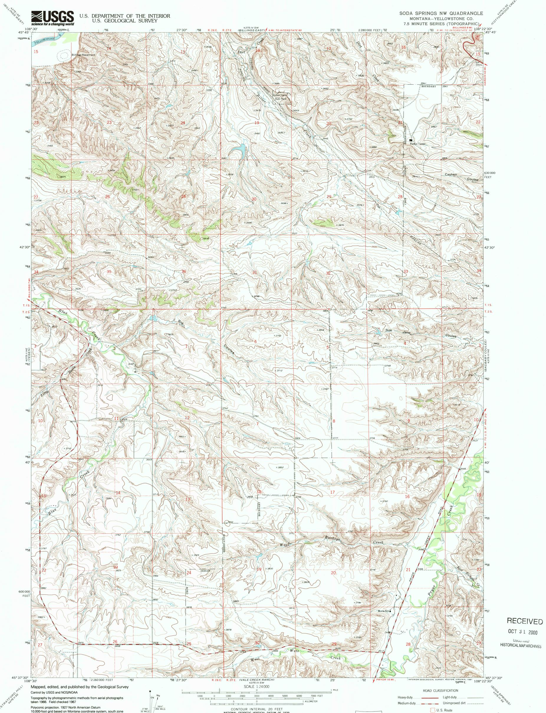
Polyconic projection. 1927 North American Datum 10,000-foot grid based on Montana coordinate system, south zone 1000-meter Universal Transverse Mercator grid ticks, zone 12 shown in blue To place on the predicted North American Datum 1983 move
