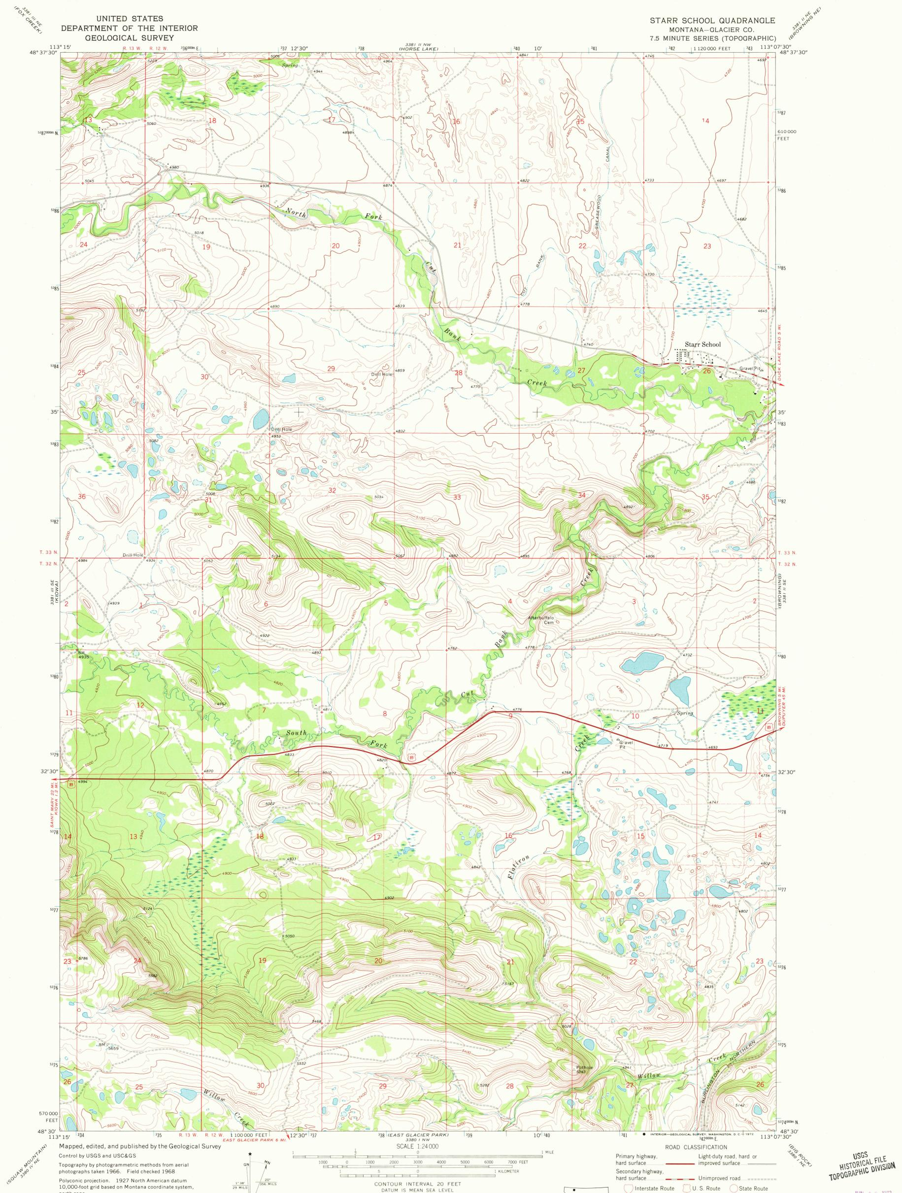
10,000-foot grid based on Montana coordinate system, north zone 1000-meter Universal Transverse Mercator grid ticks, zone 12, shown in blue UTM GRID AND 1968 MAGNETIC NORTH DECLINATION AT CENTER OF SHEET
