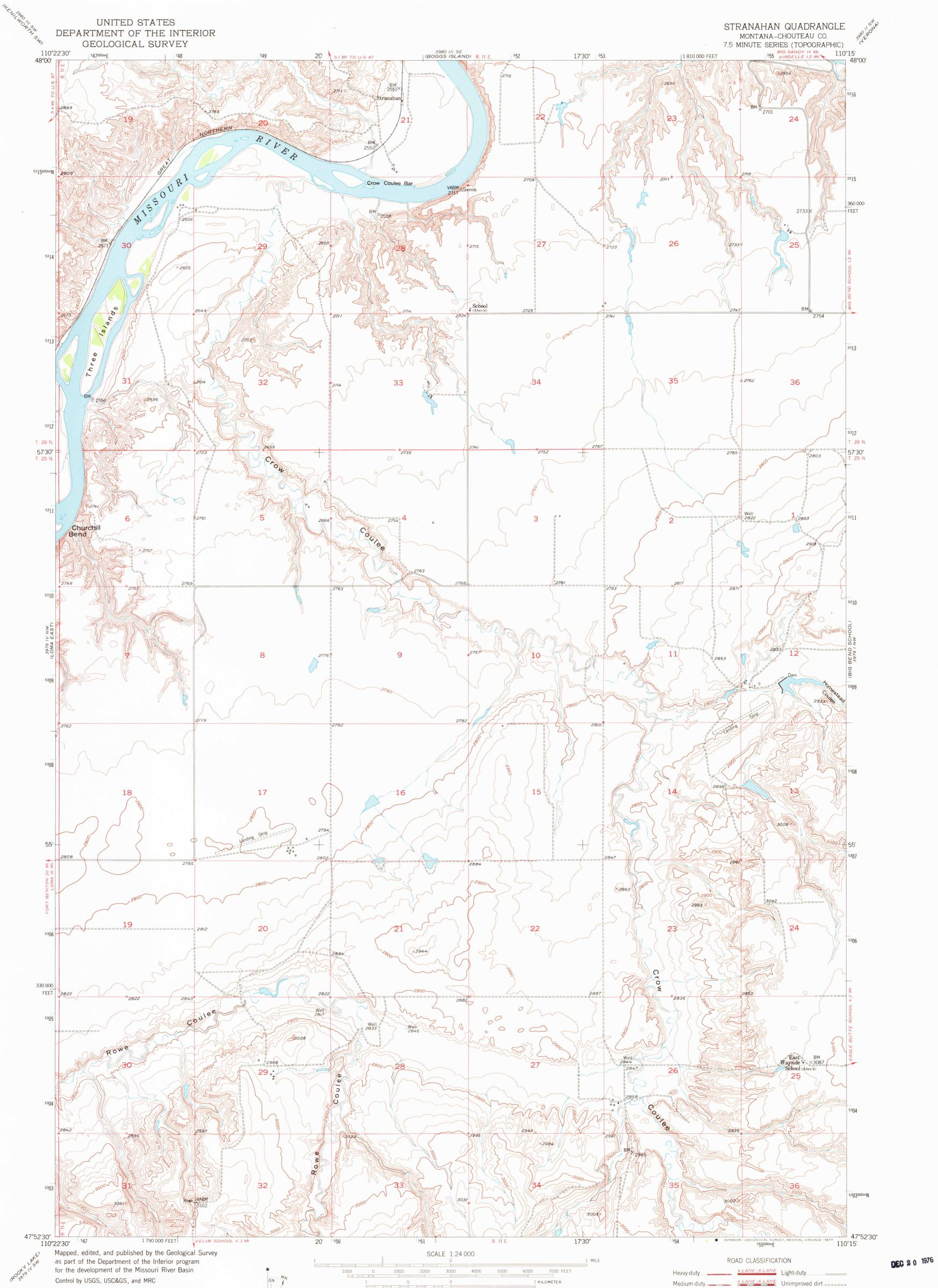
Topography from aerial photographs by multiplex methods and by plane-table surveys 1953. Aerial photographs taken 1952 Polyconic projection. 1927 North American datum 10,000-foot grid based on Montana coordinate system, north zone Dashed land lines indicate approximate locations 1000-meter Universal Transverse Mercator grid ticks, zone 12, shown in blue
