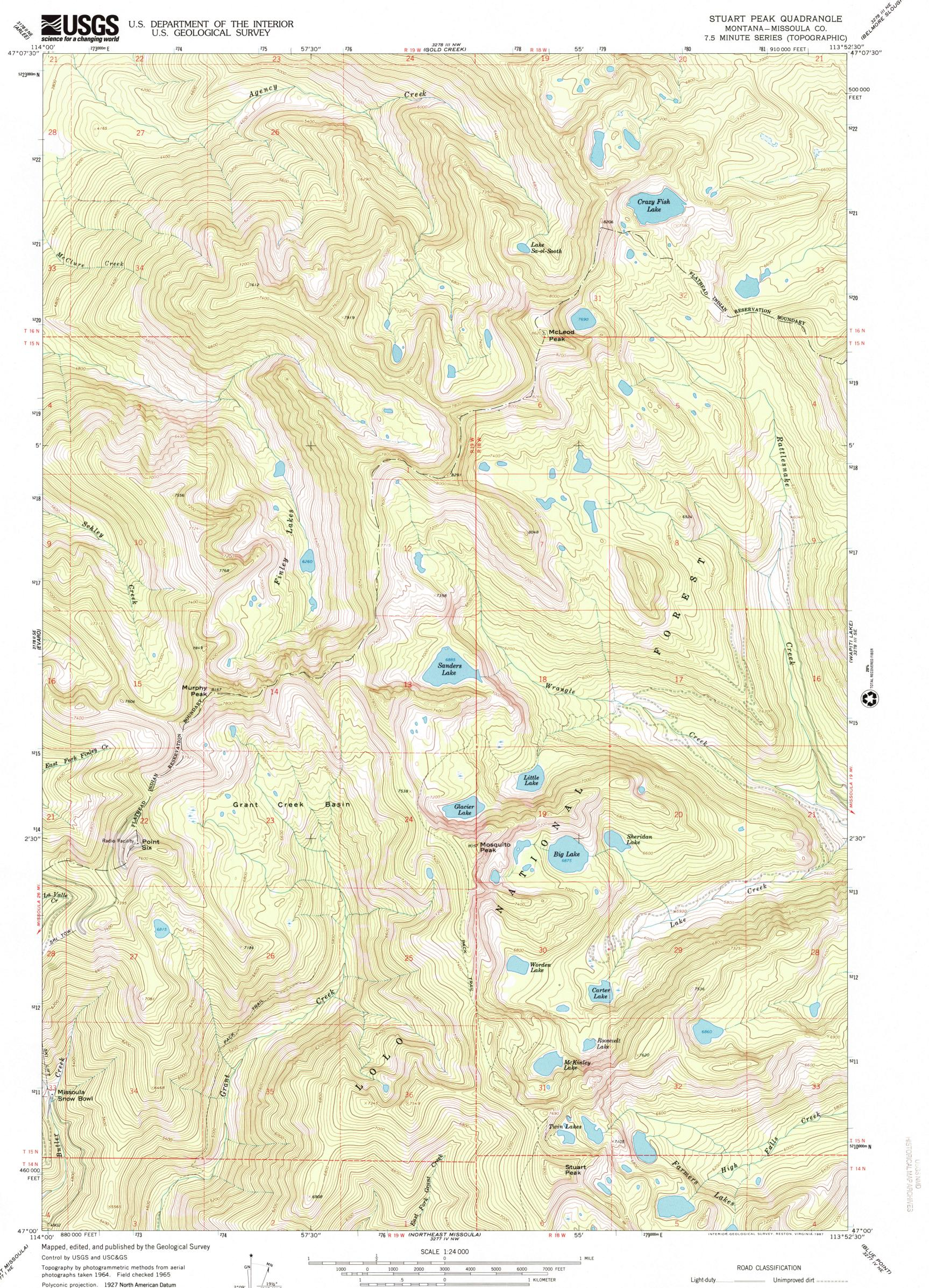
2°09' 38 MILS 10,000-foot grid based on Montana coordinate system, central zone 1000-meter Universal Transverse Mercator grid ticks, zone 12, shown in blue UTM GRID AND 1965 MAGNETIC NORTH DECLINATION AT CENTER OF SHEET Where omitted, land lines have not been established
