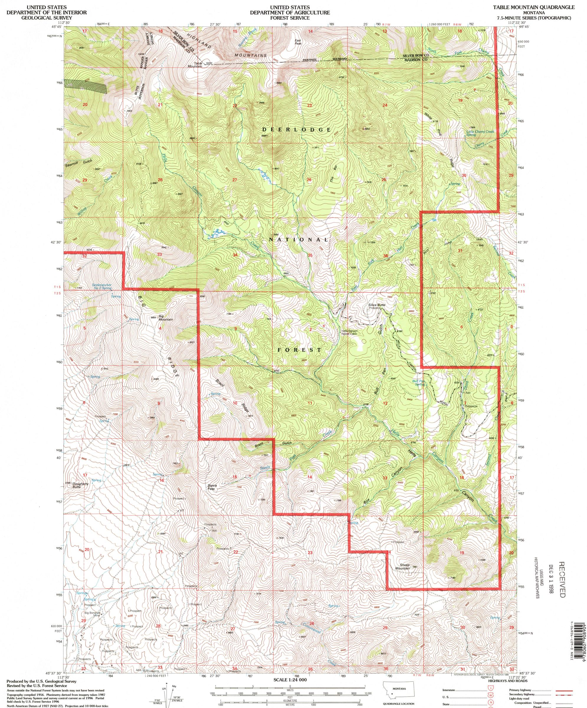
North American Datum of 1927 (NAD 27). Projection and 10 000-foot ticks: Montana coordinate system, south zone (Lambert conformal conic) Blue 1000-meter Universal Transverse Mercator ticks, zone 12 North American Datum of 1983 (NAD 83) is shown by dashed corner ticks The values of the shift between NAD 27 and NAD 83 for 7.5-minute
