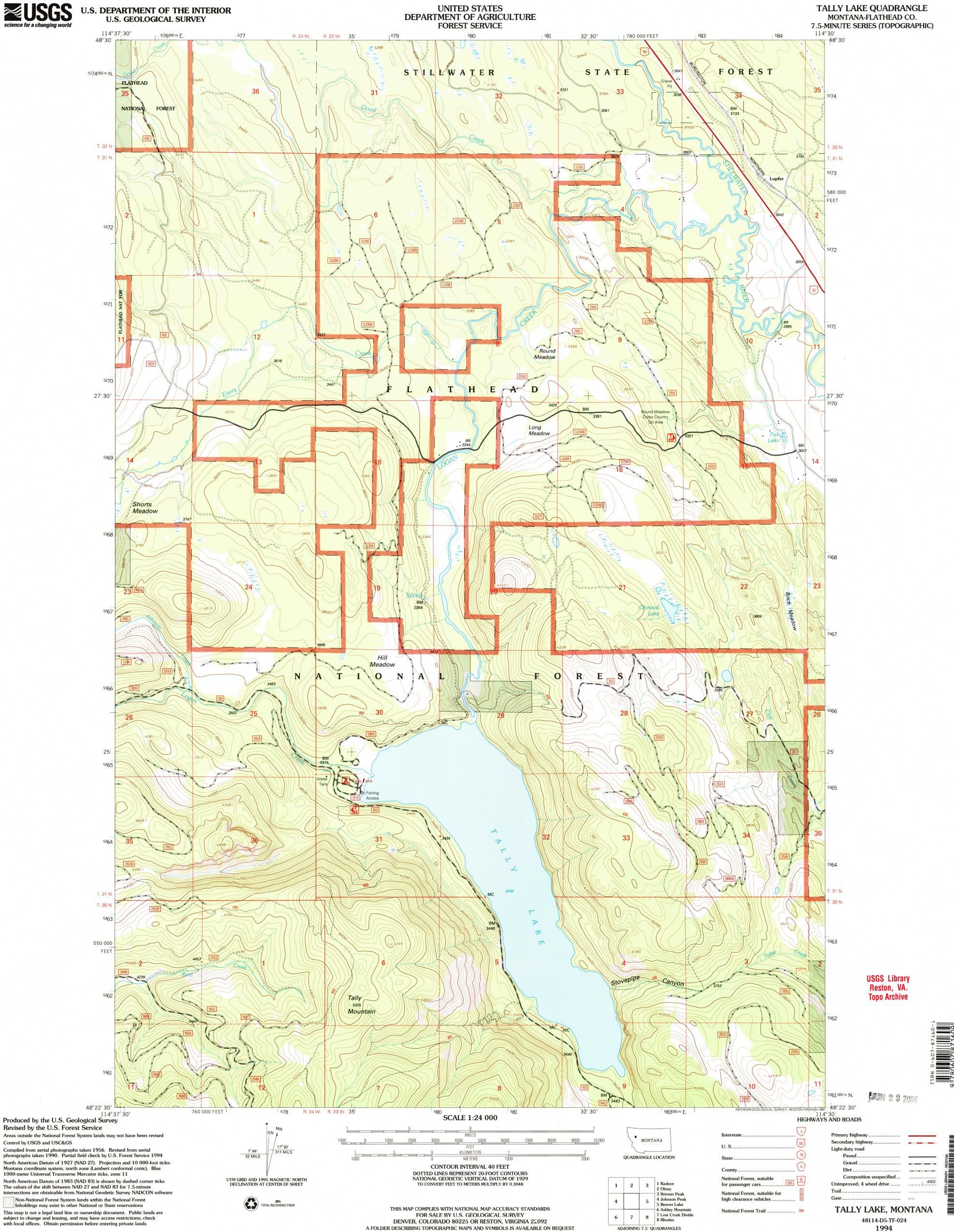
North American Datum of 1927 (NAD 27). Projection and 10 000-foot ticks: Montana coordinate system, north zone (Lambert conformal conic). Blue 1000-meter Universal Transverse Mercator ticks, zone 11
