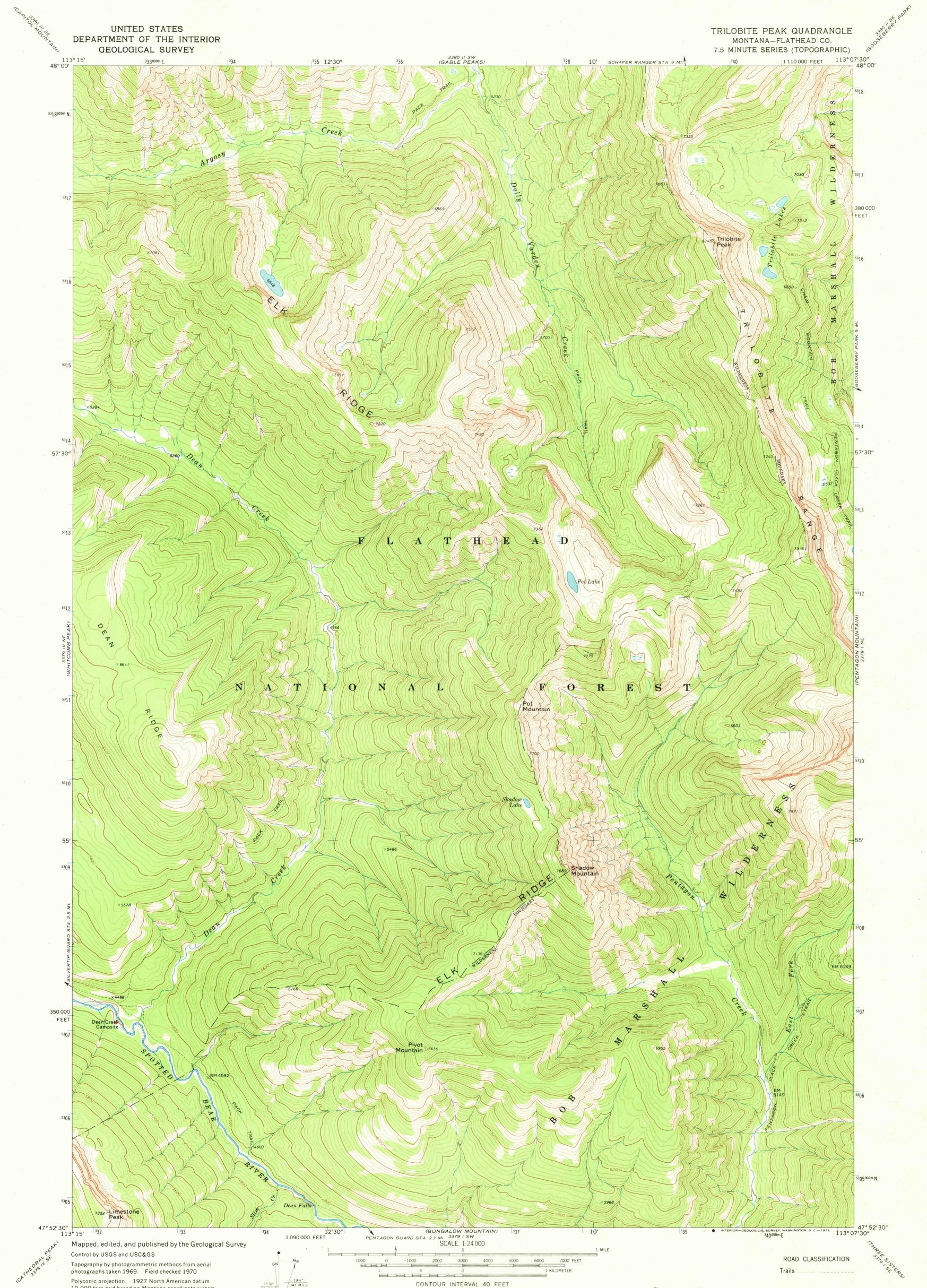
Polyconic projection. 1927 North American datum 10,000-foot grid based on Montana coordinate system, north zone 1000-meter Universal Transverse Mercator grid ticks, zone 12, shown in blue UTM GRID AND 1970 MAGNETIC NORTH DECLINATION AT CENTER OF SHEET Land lines have not been established in this area
