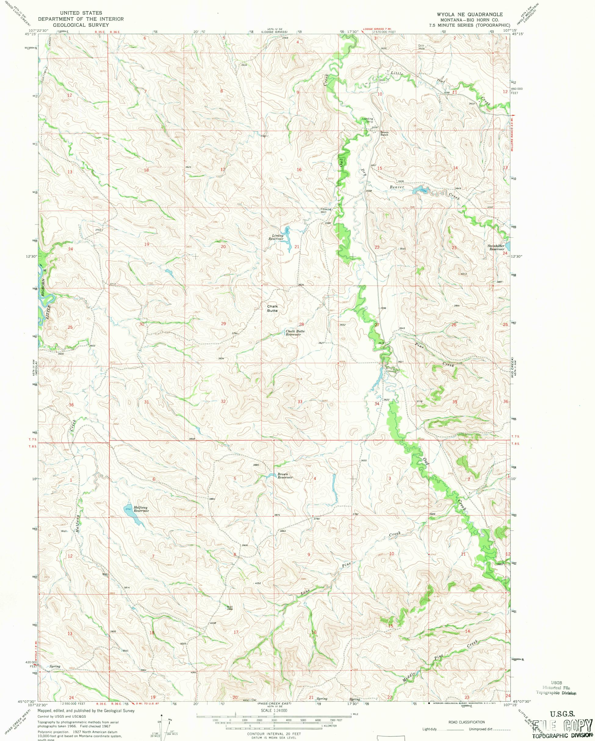
Polyconic projection. 1927 North American datum 10,000-foot grid based on Montana coordinate system, south zone 1000-meter Universal Transverse Mercator grid ticks, zone 13, shown in blue UTM GRID AND 1967 MAGNETIC NORTH DECLINATION AT CENTER OF SHEET Fine red dashed lines indicate selected fence lines Entire area lies within the boundary of the Crow Indian Reservation
