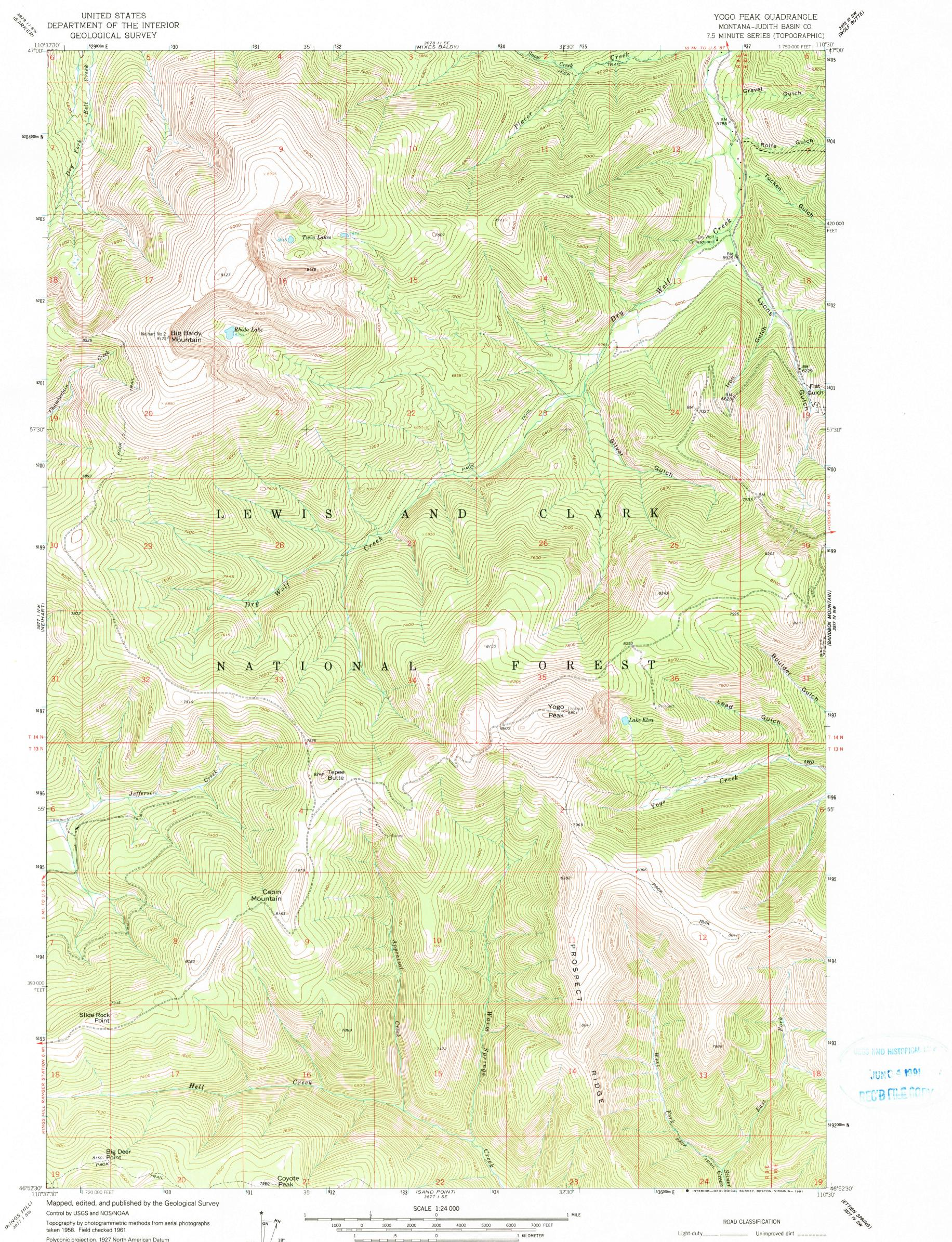
Polyconic projection. 1927 North American Datum 10,000-foot grid based on Montana coordinate system, central zone 1000-meter Universal Transverse Mercator grid ticks, zone 12 shown in blue To place on the predicted North American Datum 1983 move the projection lines 9 meters north and 60 meters east as showr by dashed corner ticks
