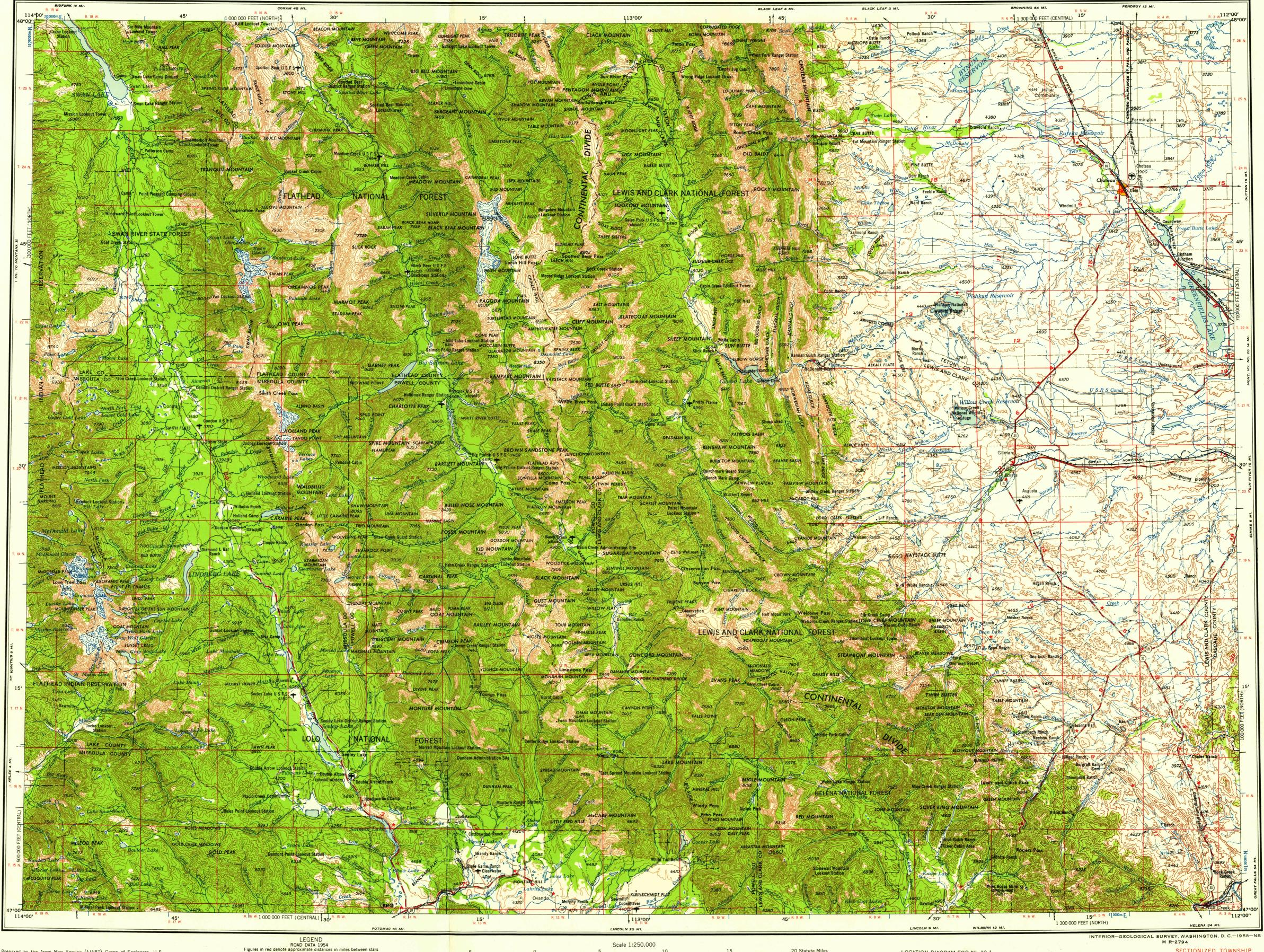
Prepared by the Army Map Service (AJART). Corps of Engineers, U.S. Army, Washington, D.C. Compiled in 1955 by photogrammetric methods. Horizontal and vertical control by USGS, USC&GS and CE. Aerial photog-raphy 1953. Photography field annotated in 1954. 100,000 foot grids based on Montana coordinate system, central and north zones 10,000-meter Universal Transverse Mercator grid ticks, zone 12, shown in blue
