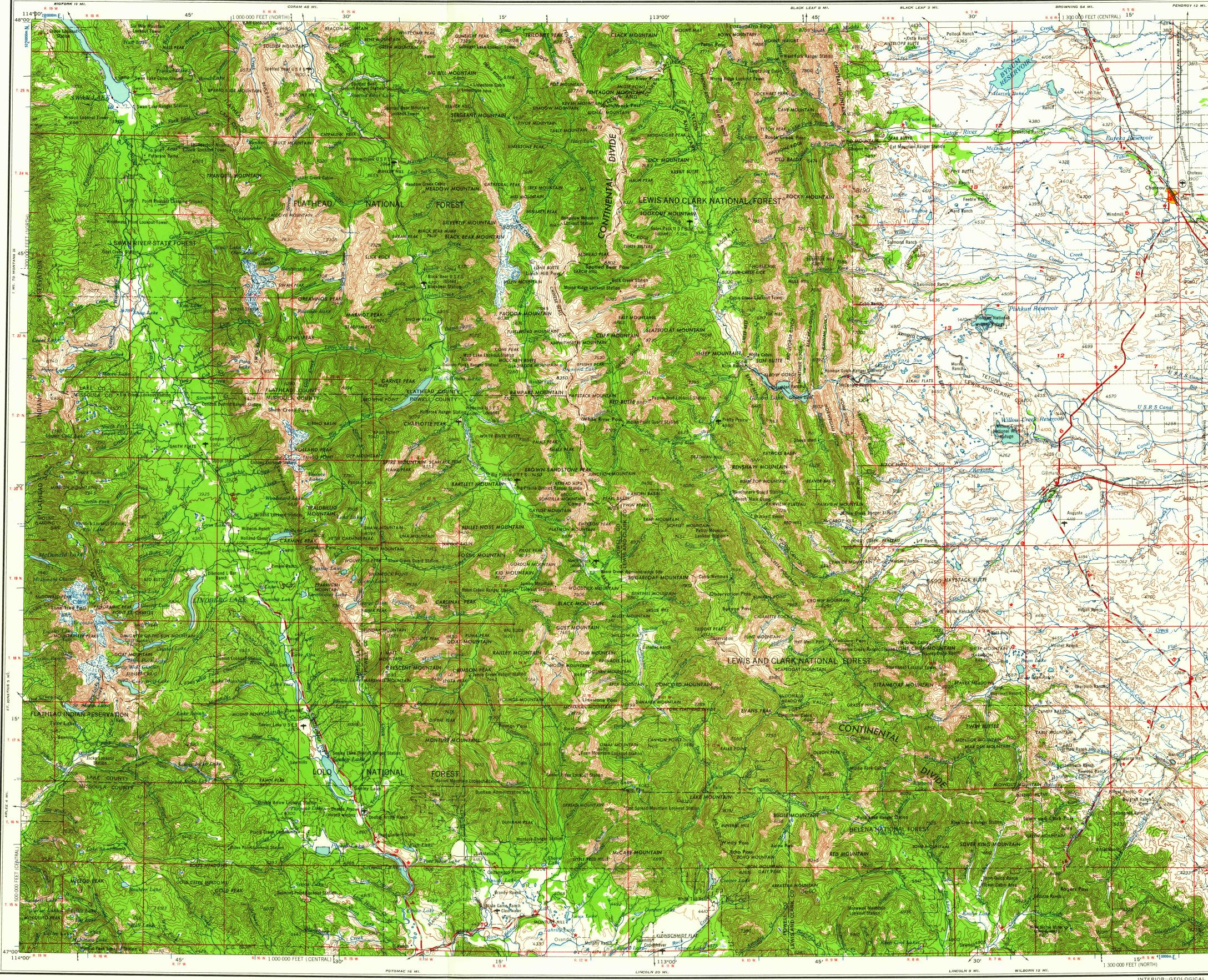
Prepared by the Army Map Service (AJART). Corps of Engineers, U.S. Army, Washington, D.C. Compiled in 1955 by photogrammetric methods. Horizontal and vertical control by USGS, USC&GS and CE. Aerial photog-raphy 1953. Photography field annotated in 1954. 100,000 foot grids based on Montana coordinate system, central and north zones 10,000-meter Universal Transverse Mercator grid ticks, zone 12, shown in blue
