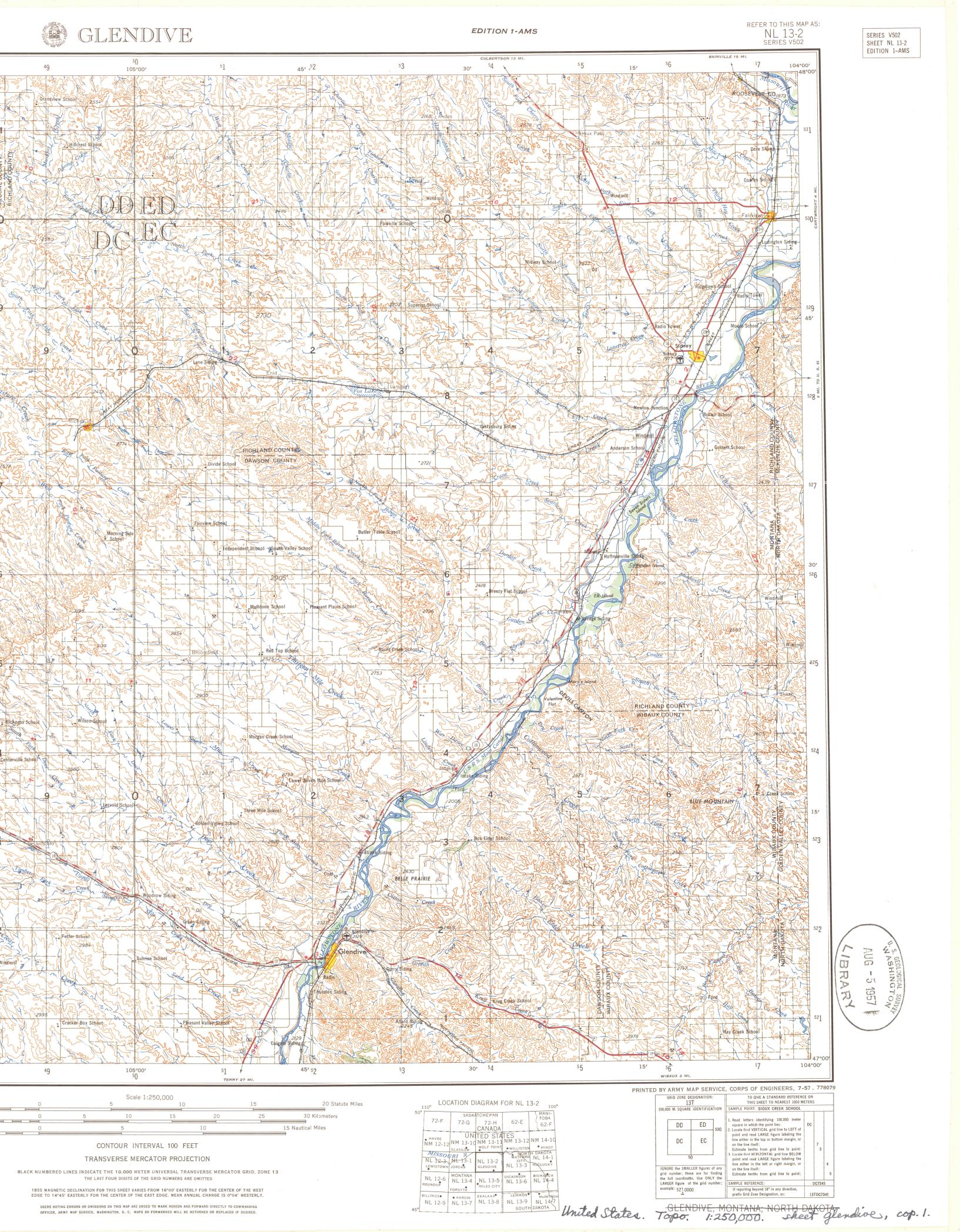
BLACK NUMBERED LINES INDICATE THE 10,000 METER UNIVERSAL TRANSVERSE MERCATOR GRID, ZONE 13 1955 MAGNETIC DECLINATION FOR THIS SHEET VARIES FROM 16°00' EASTERLY FOR THE CENTER OF THE WEST EDGE TO 14°45' EASTERLY FOR THE CENTER OF THE EAST EDGE. MEAN ANNUAL CHANGE IS 0°04' WESTERLY.
