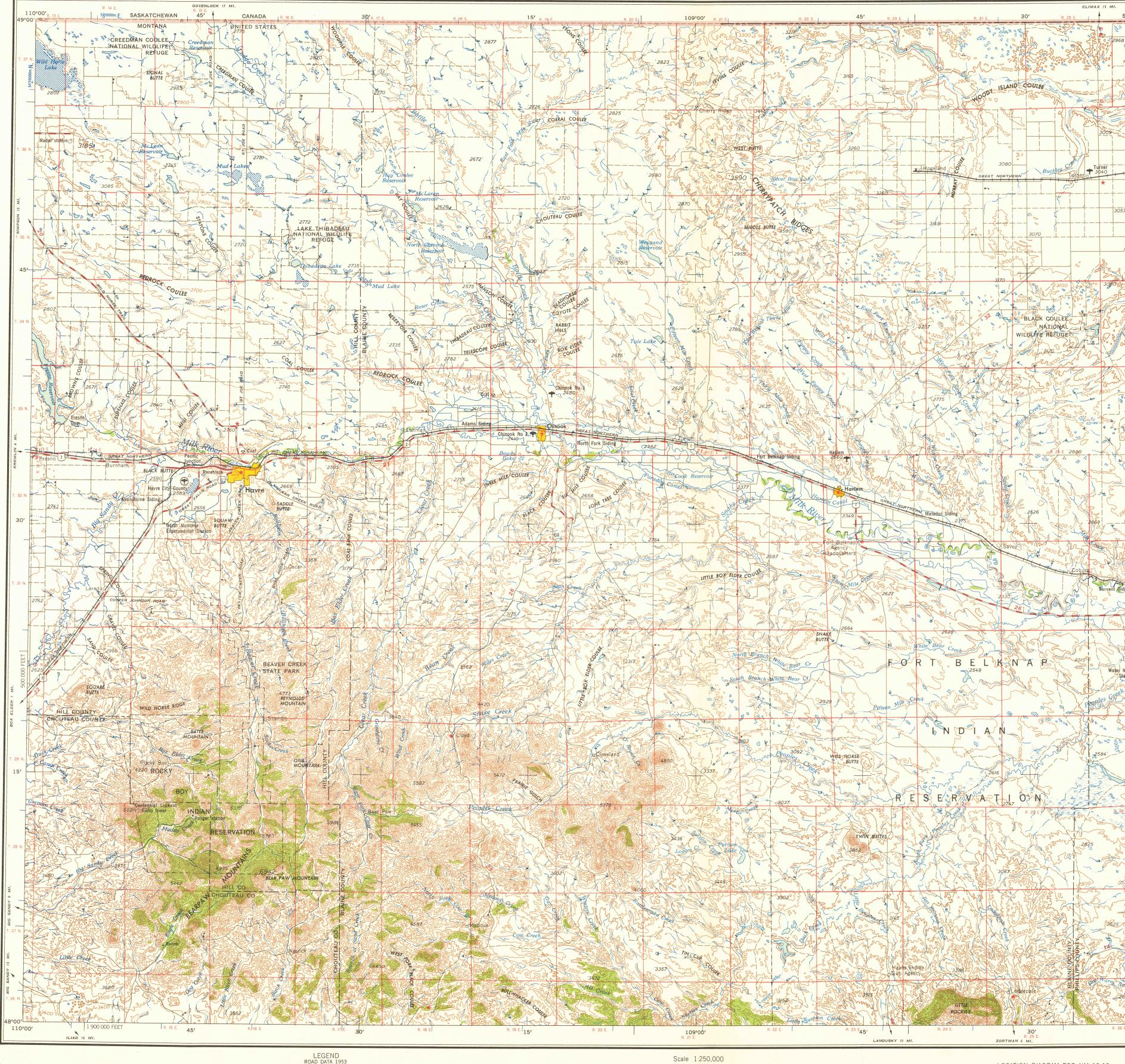
Prepared by the Army Map Service (ASSX), Corps of Engineers, U.S. Army, Washington, D.C. Compiled in 1955 by photogrammetric methods. Horizontal and vertical control by USC&GS, USGS and IBC. Aerial photography 1952. Photography field annotated 1953. Over 100,000-foot grids based on Montana coordinate system north zone 100, 10,000-meter Universal Transverse Mercator grid ticks, zone 12, shown in blue 5,00
