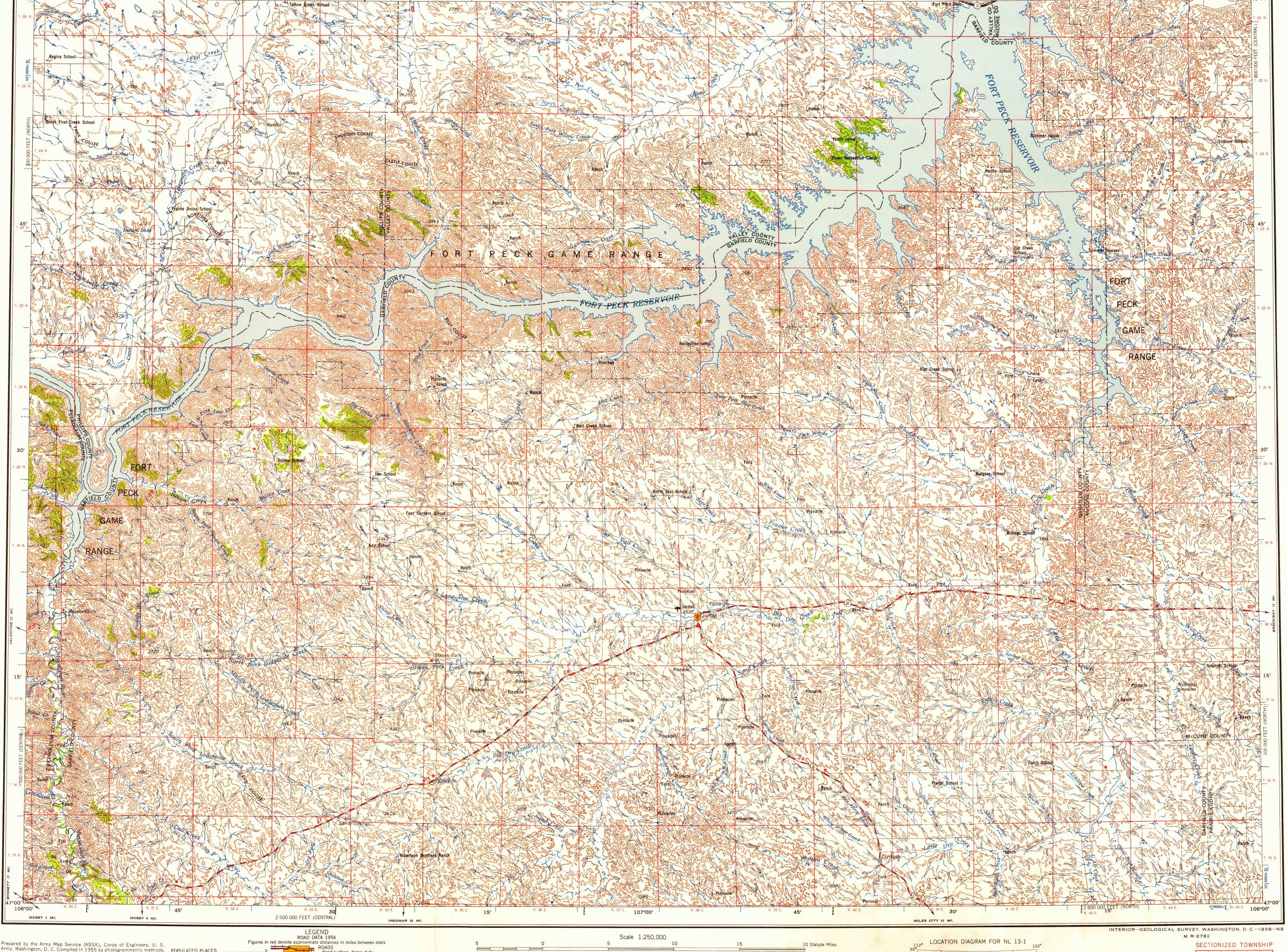
Prepared by the Army Map Service (ASSX), Corps of Engineers, U. S. Army, Washington, D. C. Compiled in 1955 by photogrammetric methods. Horizontal and vertical control by USC&GS, USGS and CE. Aerial photography 1951-52. Photography field annotated 1954.
