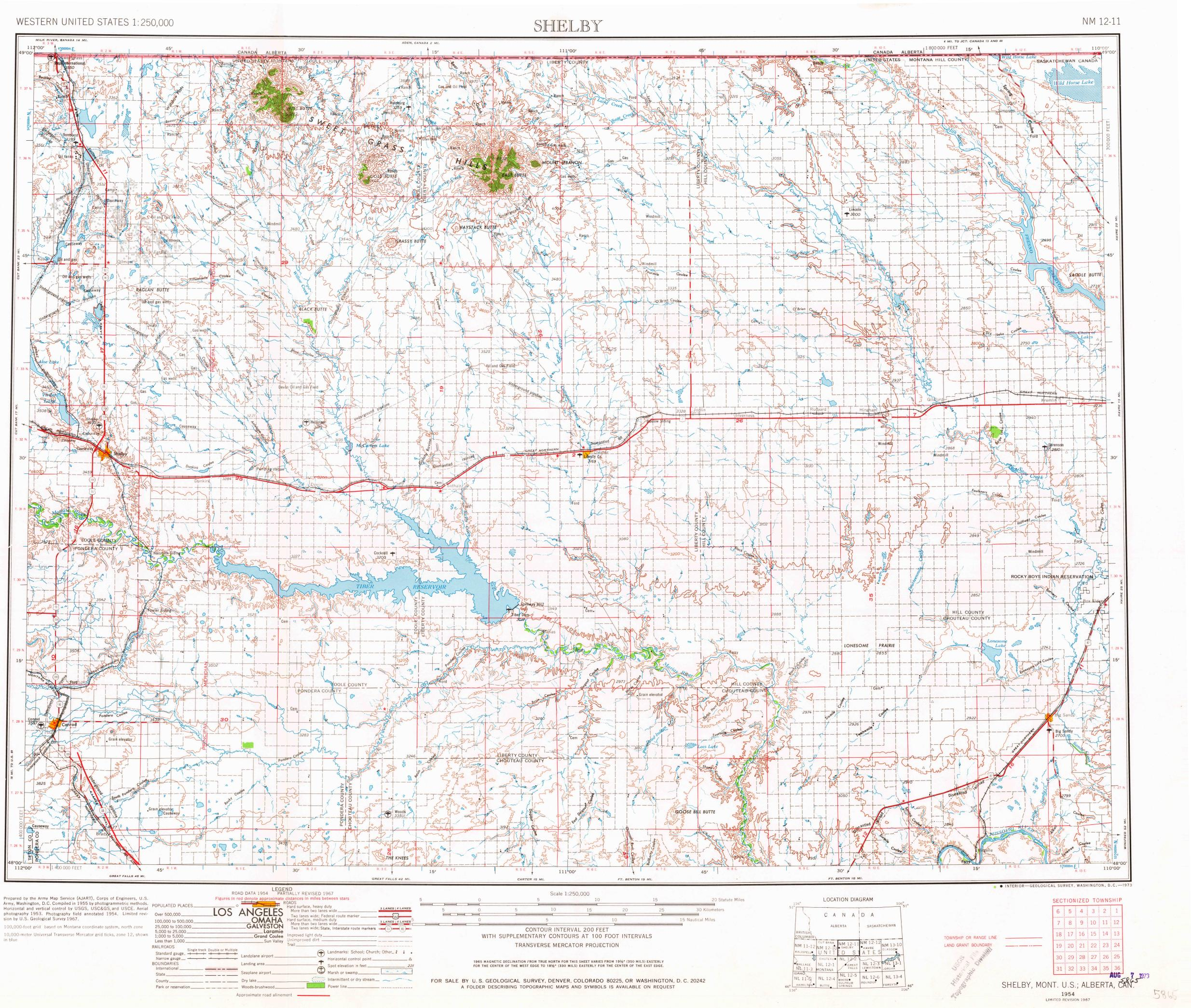
Prepared by the Army Map Service (AJART), Corps of Engineers, U.S. Army, Washington, D.C. Compiled in 1955 by photogrammetric methods. Horizontal and vertical control by USGS, USC&GS, and USCE. Aerial photography 1953. Photography field annotated 1954. Limited revision by U.S. Geological Survey 1967. 100,000-foot grid based on Montana coordinate system, north zone
