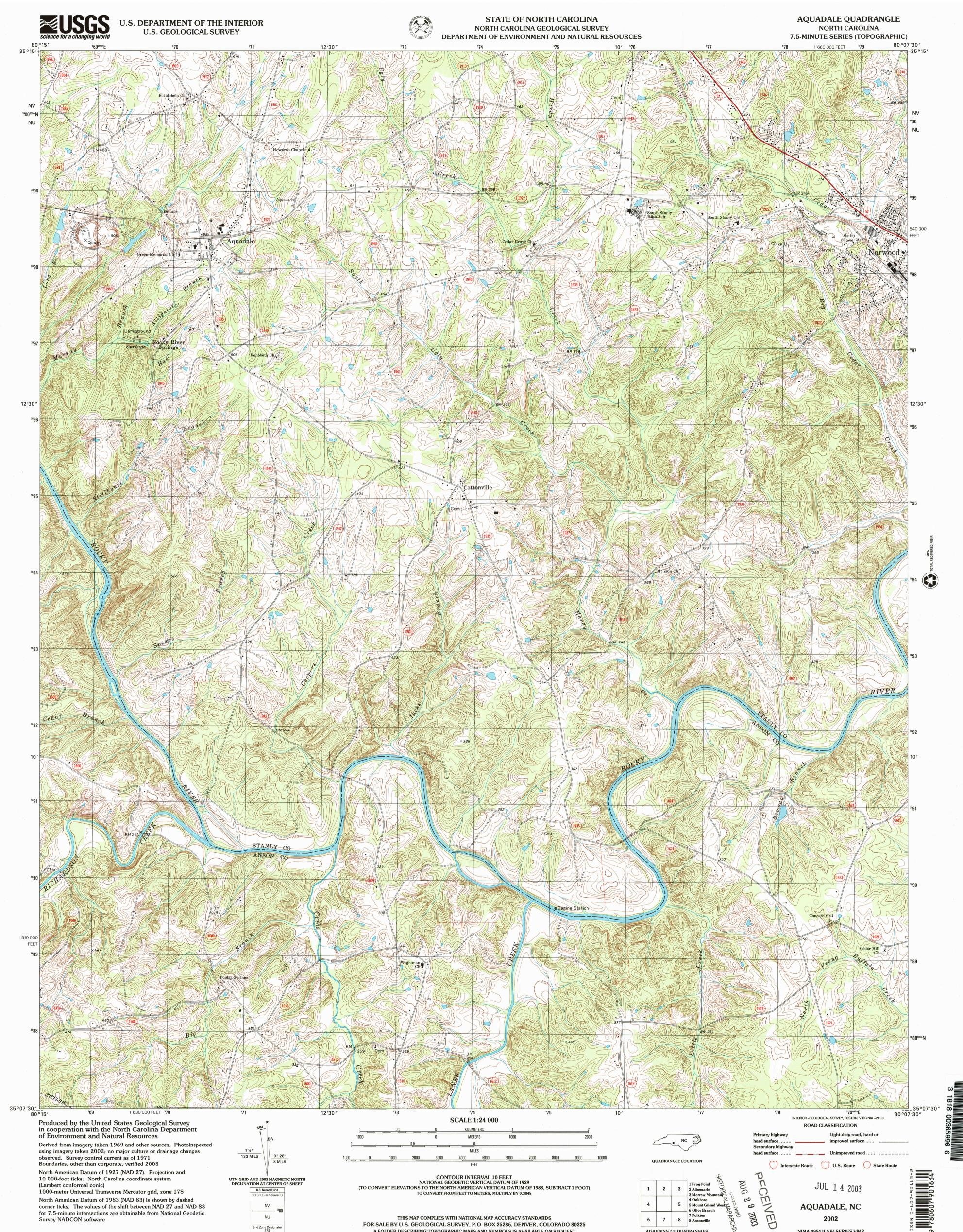
North American Datum of 1927 (NAD 27). Projection and 10 000-foot ticks: North Carolina coordinate system (Lambert conformal conic) 1000-meter Universal Transverse Mercator grid, zone 17S North American Datum of 1983 (NAD 83) is shown by dashed corner ticks. The values of the shift between NAD 27 and NAD 83 for 7.5-minute intersections are obtainable from National Geodetic Survey NADCON software
